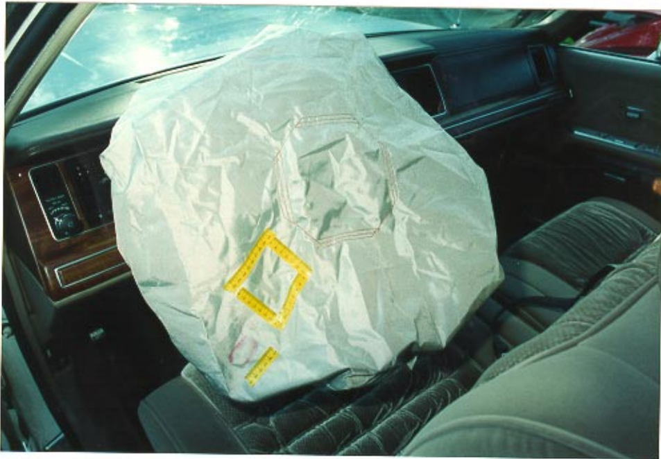
23. Overall view of the deployed driver's side air bag.
