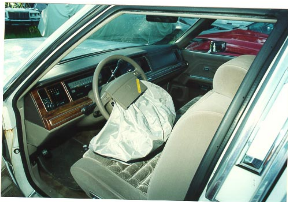
20. Overall interior view and the deployed driver's side air bag.
