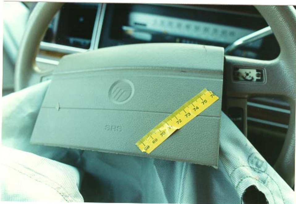
26. Probable area of contact with the driver's right forearm.
