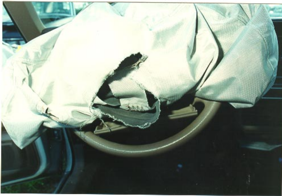
30. Tear of the air bag membrane at the 6 o'clock position of the air bag.
