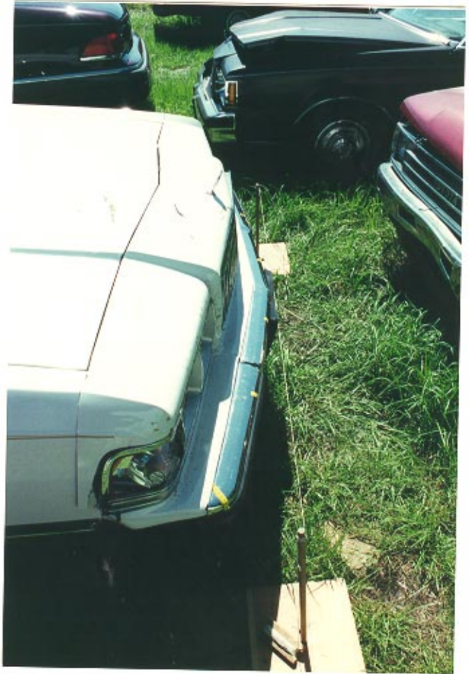
13. & 14. Profile views of the frontal area showing the minor severity impact damage.
