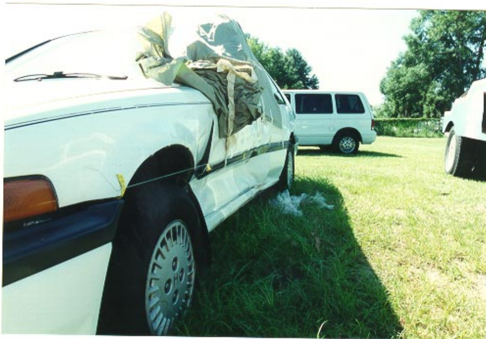
43. Longitudinal view documenting the extent of side crush.
