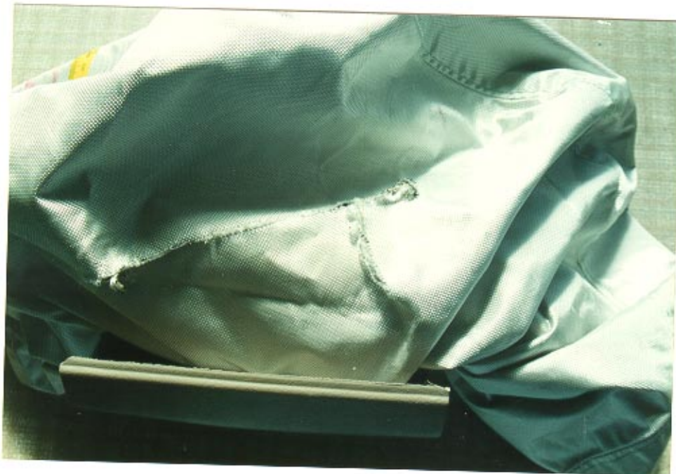
32. T-shaped tear pattern.
