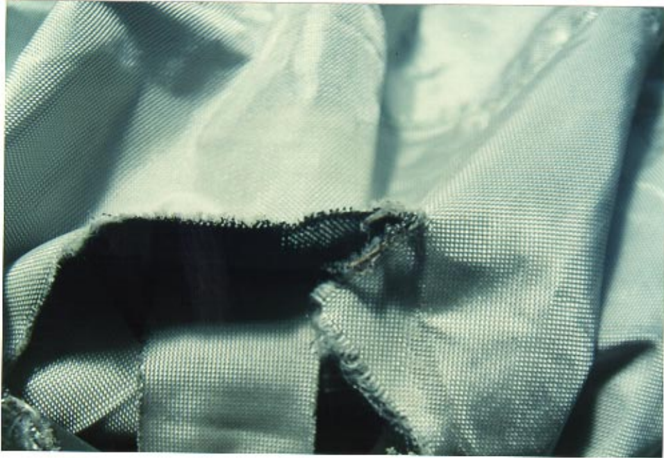
35. Close-up view of the edges of the tear.
