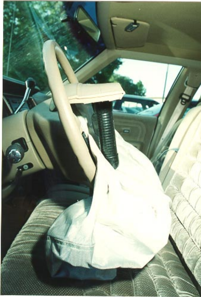
27. Perpendicular view of the upper module cover flap.
