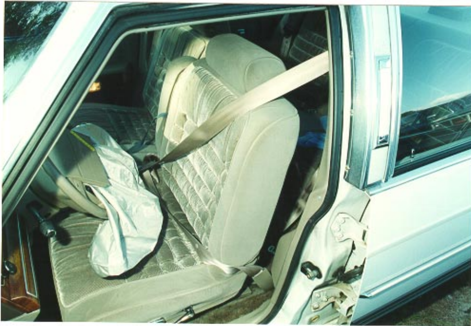
21. Driver's seat track adjustment and the 3-point lap and shoulder belt system.
