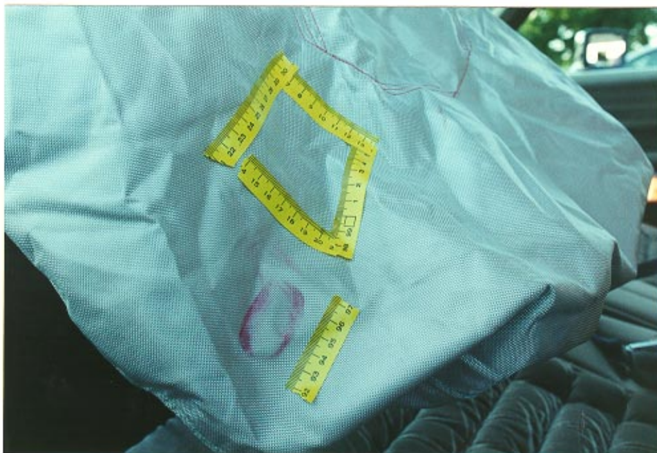
24. Driver lipstick transfer to the lower left quadrant of the air bag.
