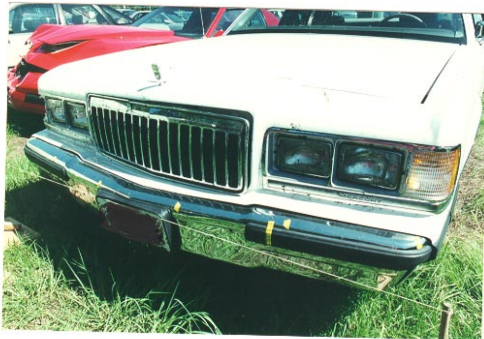
9. & 10. Minor impact damage to the frontal area of the Grand Marquis.
