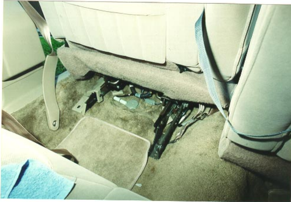
39. Exposed driver's side seat track into the left rear area with the seat adjusted to a forward track position.
