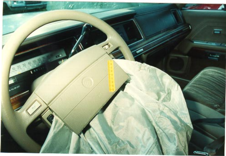
25. Asymmetrical upper air bag module cover flap.
