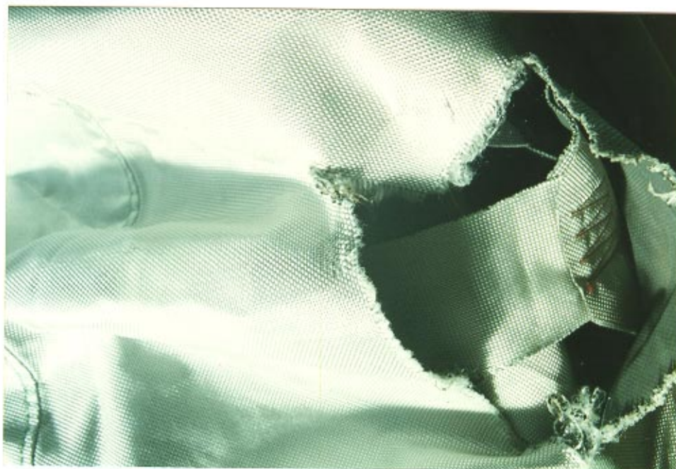
34. Close-up view of the tear at the right edge.
