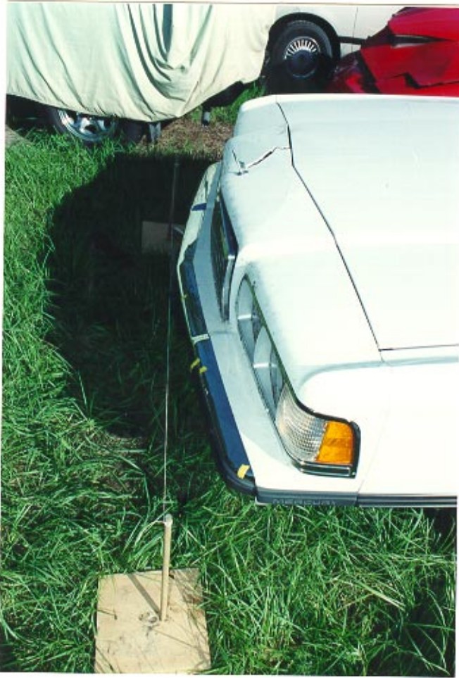
13. & 14. Profile views of the frontal area showing the minor severity impact damage.
