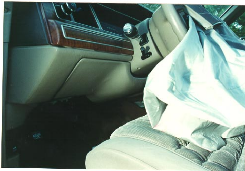
22. Close proximity of the driver's seat to the knee bolster.
