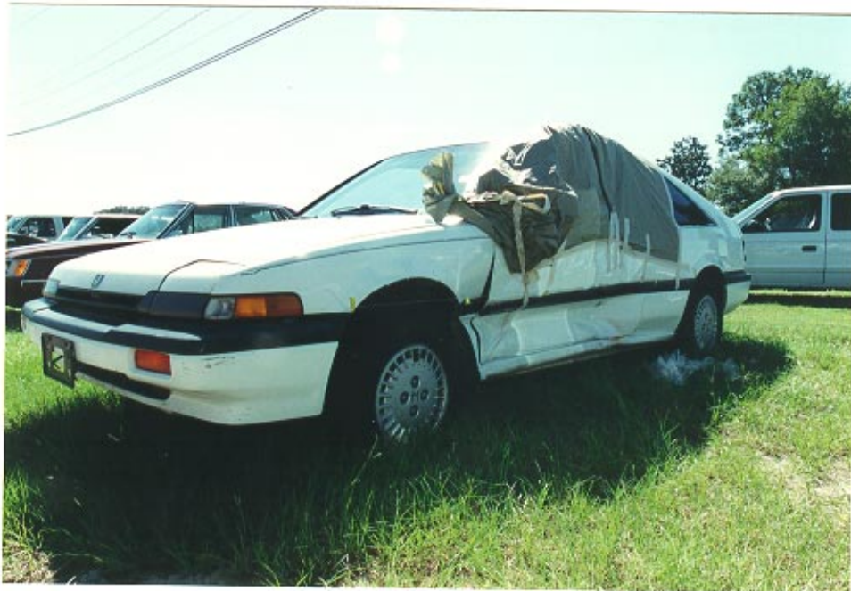
42. Impact damage to the left side area of the struck Honda Accord.
