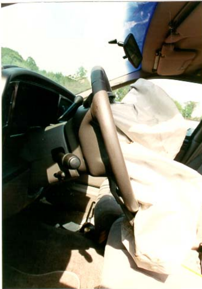
22. Profile view of the steering wheel; no deformation.
