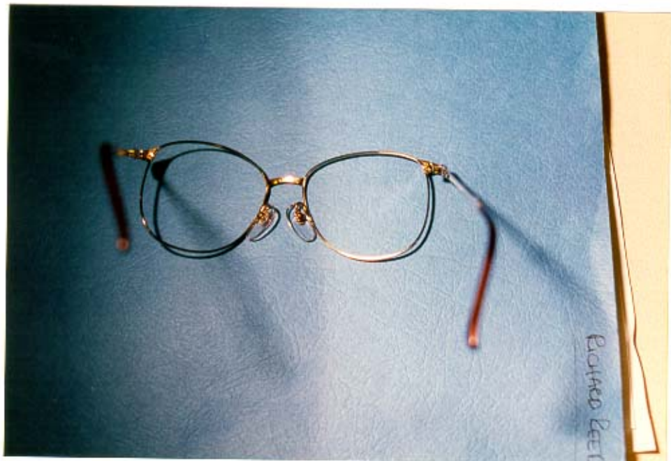
30. Deformed eyeglass frames from air bag involvement.
