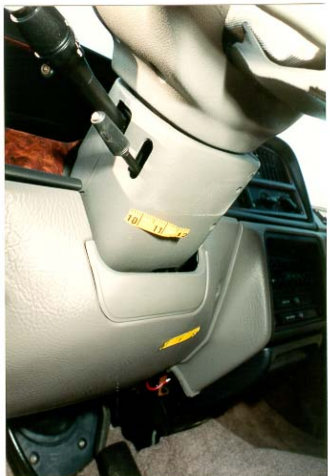
24. Driver knee loading to the steering column cover and bolster.
