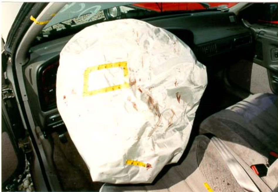
18. Driver contact points on the deployed air bag.
