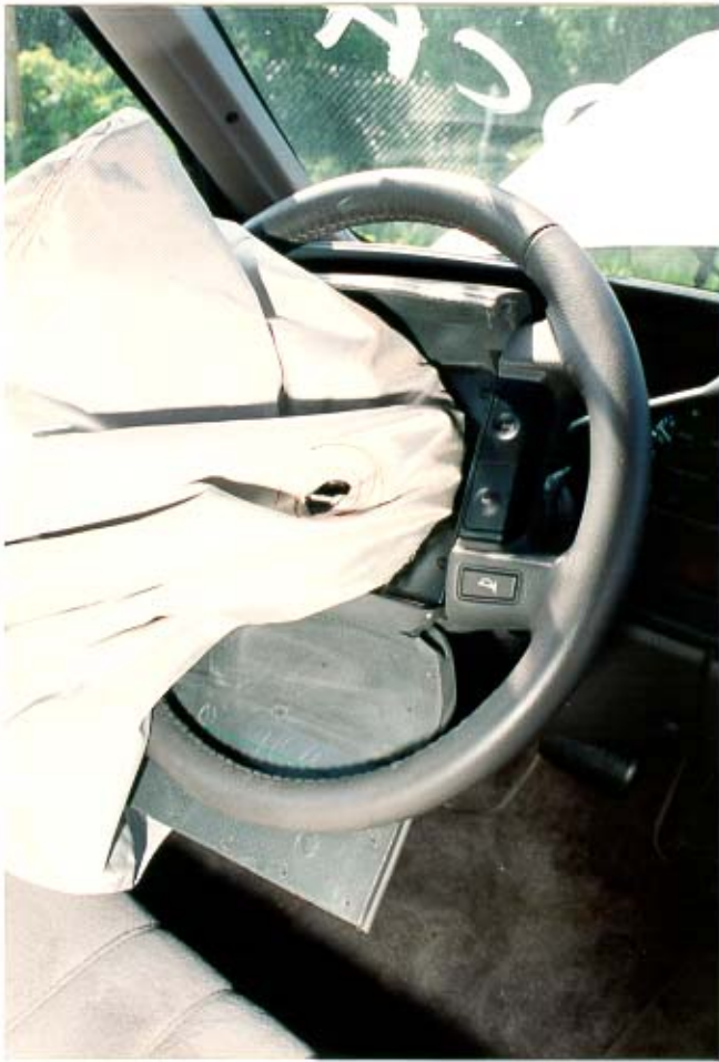
23. Air bag vent port and module cover flap configuration (wheel rotated 180 degrees).
