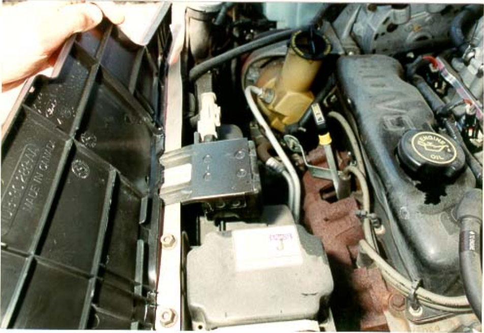
15. Center front air bag crash sensor.
