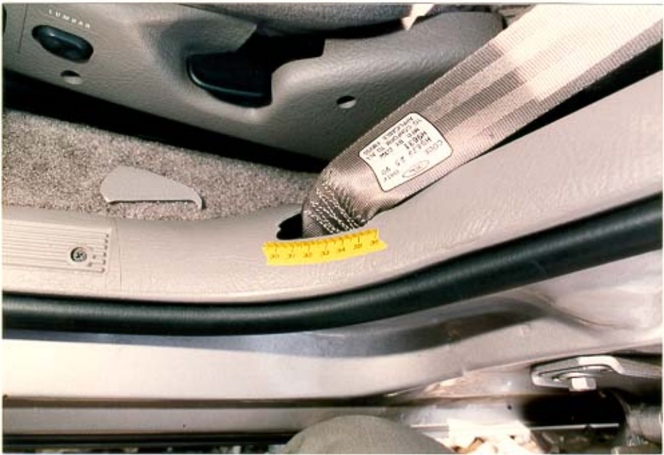
21. Belt loading fracture to the plastic sill trim.
