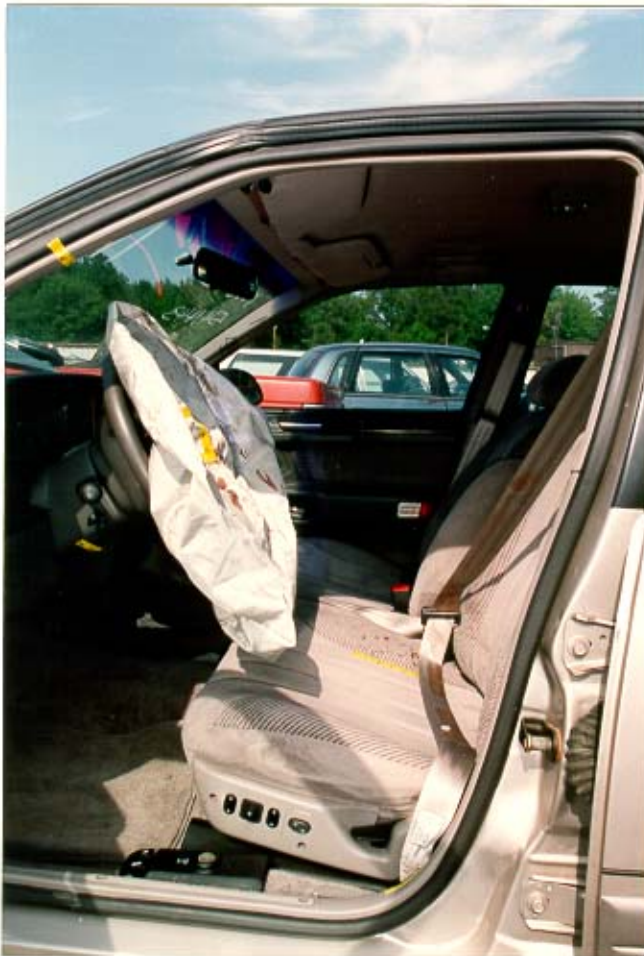
17. Overall view of the driver's compartment and the deployed air bag.
