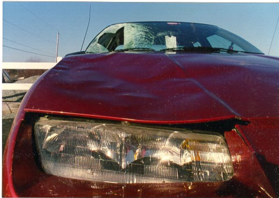
26. Close-up view along hood edge line providing more definition on contact points and vertical crush.
