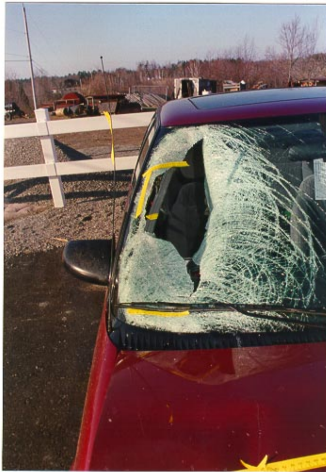
35. View of windshield showing pedestrian contact points.
