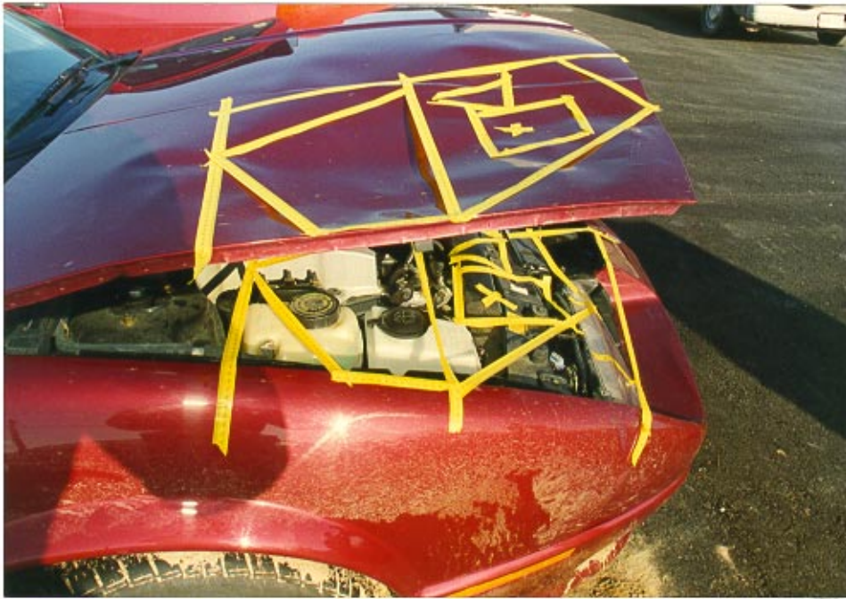
37. Lateral view of hood contact evidence showing an overlay mapping of pedestrian contact points with underlying engine compartment components.
