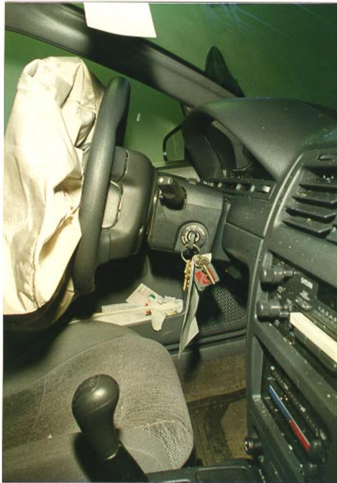
57. Lateral view of steering wheel and steering column verifying no rim displacement.
