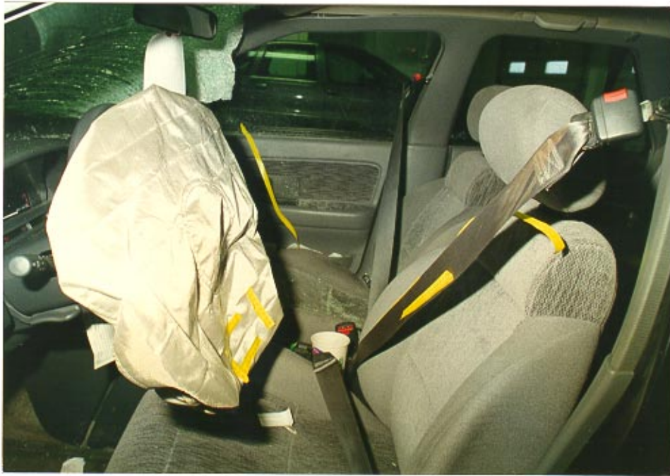
43. Lateral view of front seating area taken from the left side of the vehicle showing contact evidence on the shoulder belt and right front door surface.
