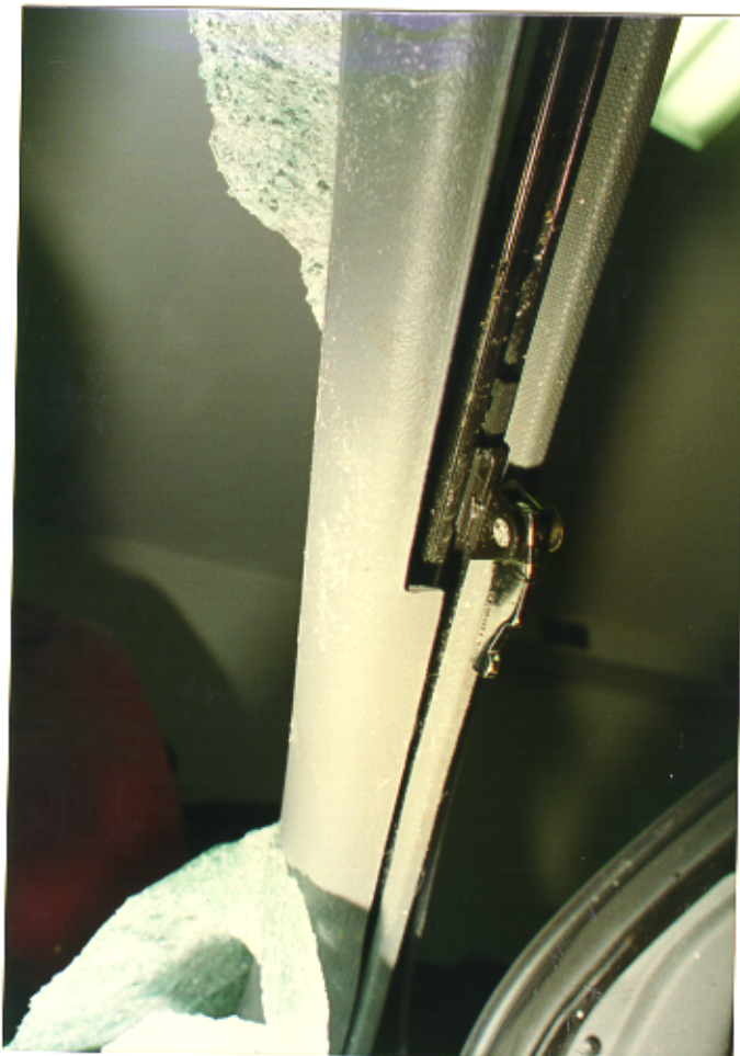
52. Close-up view of contact by the pedestrian's head on the right A-pillar cover.
