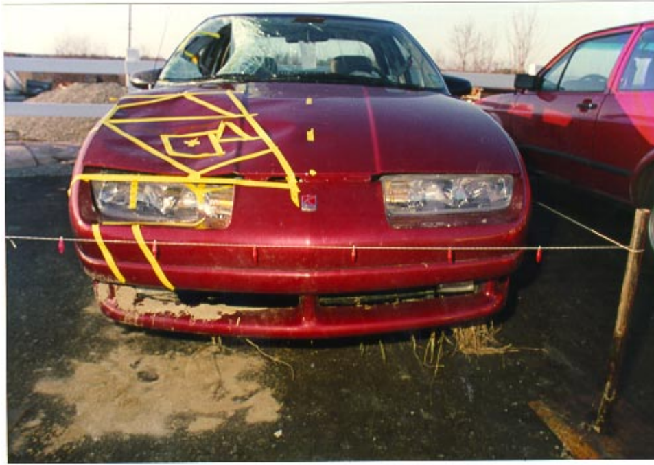
29. Frontal view with calibrated tape applied. The box with the "X" indicates a focal point from hip contact while the triangular area highlights the contact point by the pedestrian's right elbow.
