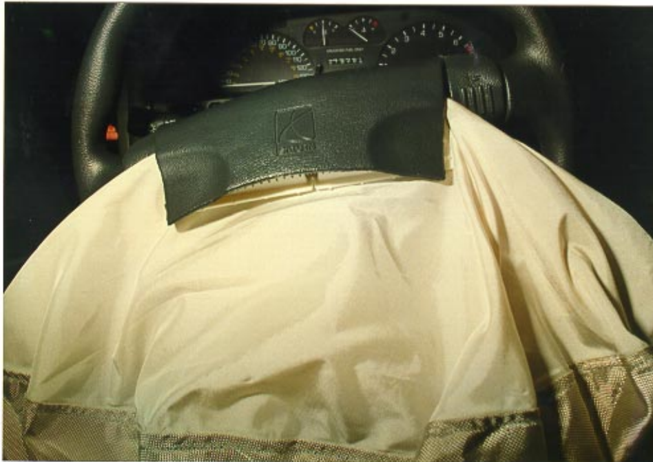
48. View of the upper flap of the air bag module cover.
