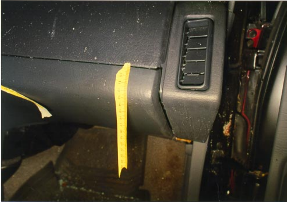
53. Close-up view of a right knee contact by the right front passenger along the lower edge of the instrument panel
