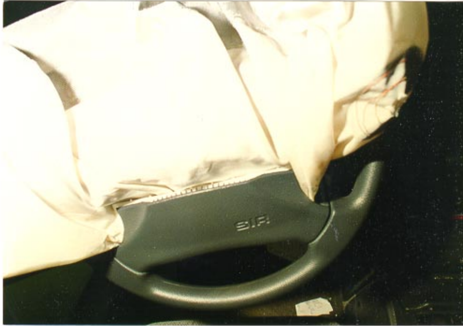
49. View of lower flap of the air bag module cover.
