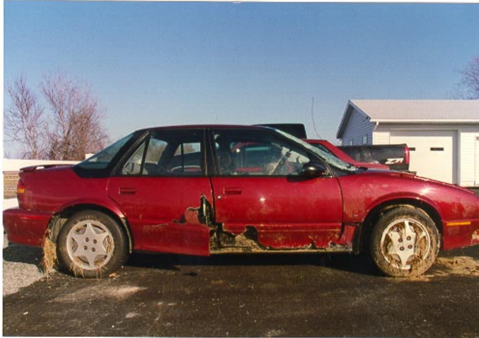
41. View of right side plane showing contact damage from utility pole guy wire and ditch.
