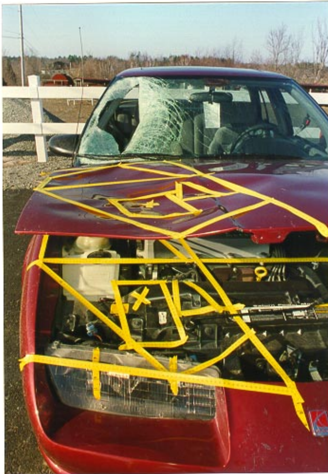
32. Bi-level view of the hood contact pattern and corresponding underhood components.
