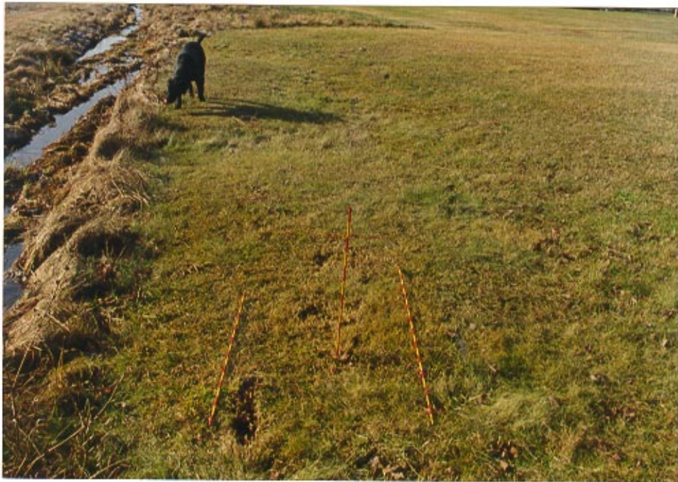
11. Close-up of lawn contact by pedestrian, with gouging and grass scuffing in the direction of the pedestrian's trajectory.
