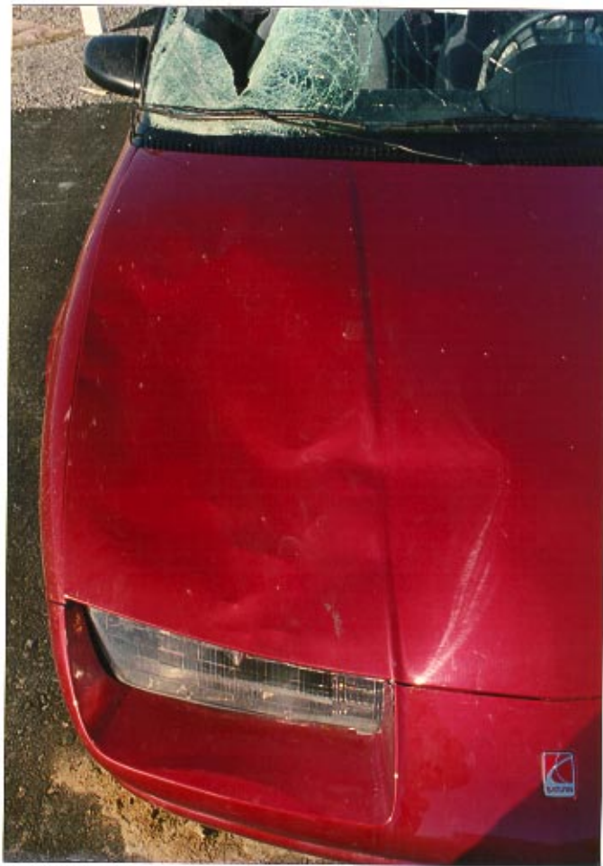
27. Overhead view of contact pattern on hood prior to highlighting with calibrated tape.
