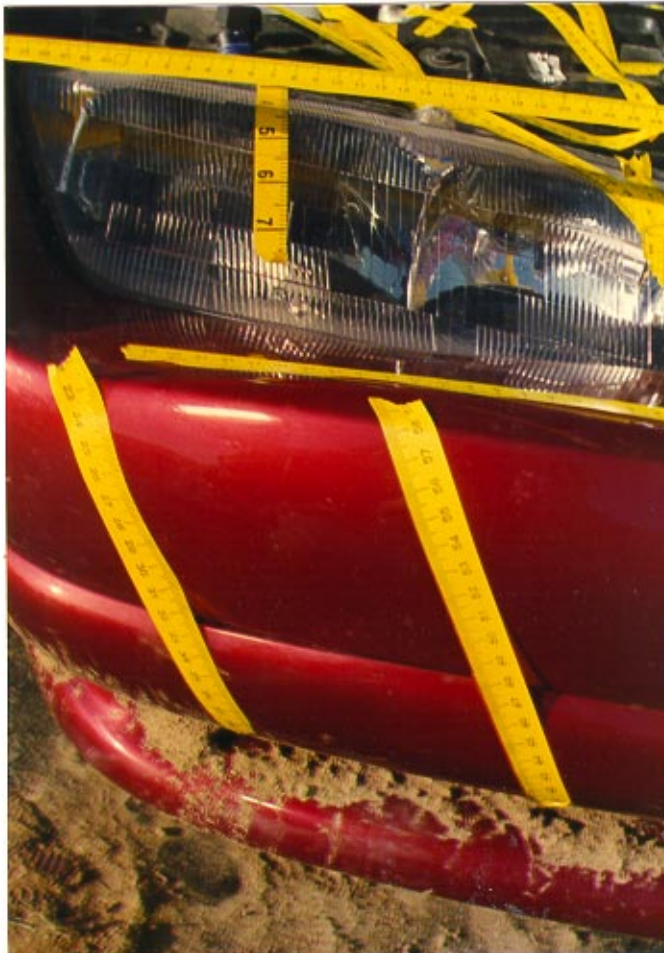
30. Close-up view of the right front bumper face highlighting the left leg contact pattern.
