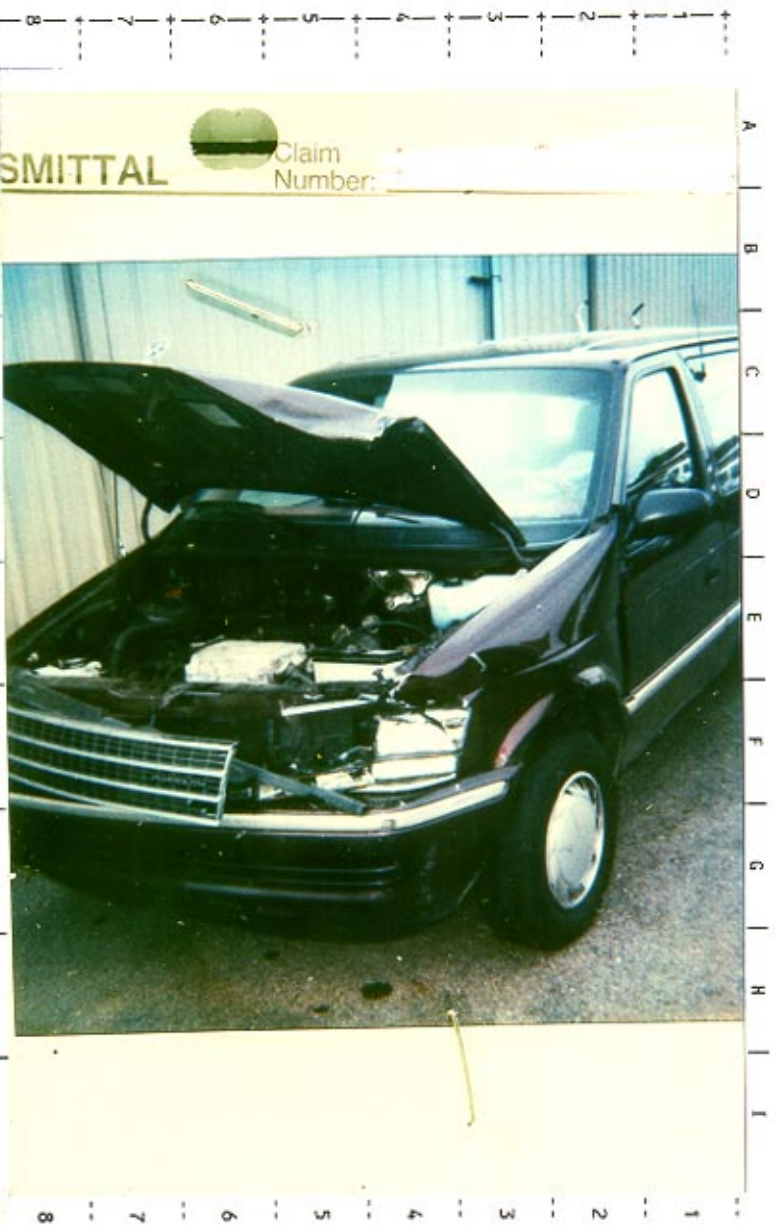
# 01 -- 1993 Plymouth Voyager viewed from front left showing impact at front left corner; NOTE: majority of damage is above bumper
