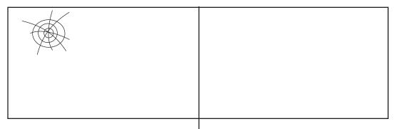
Windshield cracked on upper left, possibly due to contact by the driver
