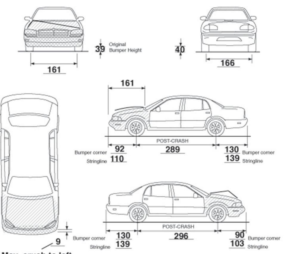
Max. crush to left front bumper corner
