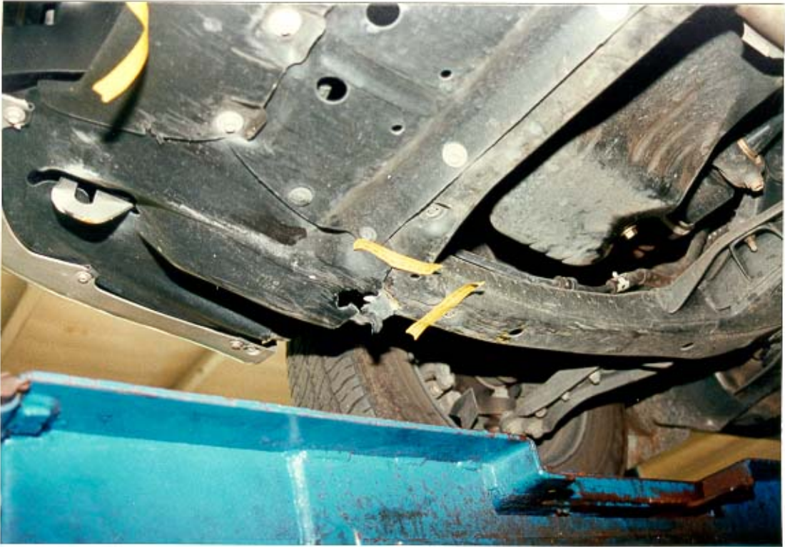
Damage to splash panel and frame
