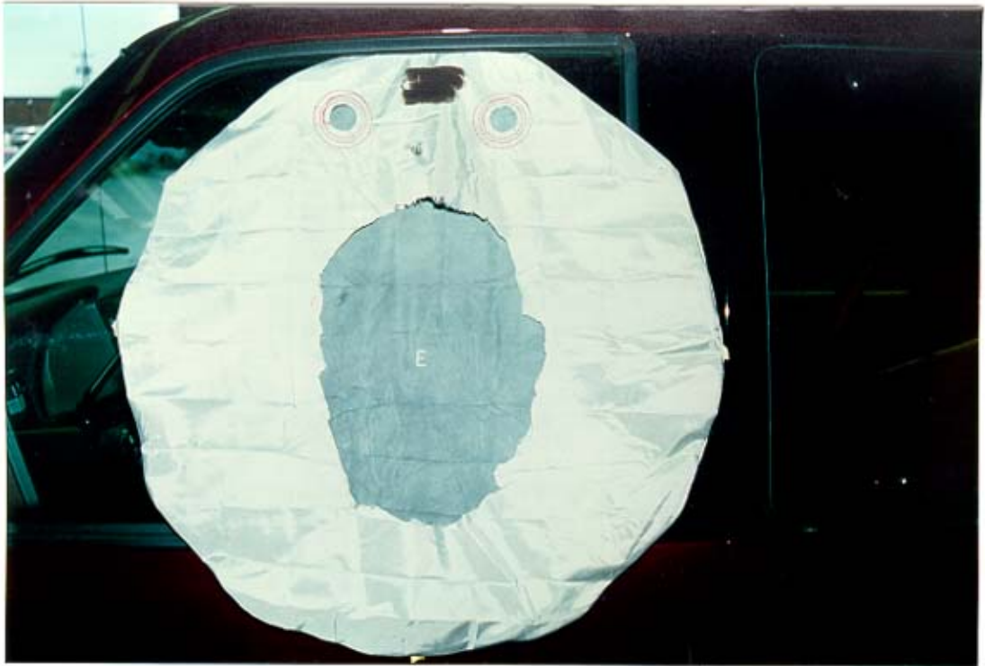
Reverse side of airbag (note vent ports are at top position of airbag)
