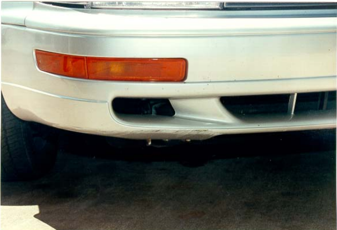
Closeup of damage to fascia
