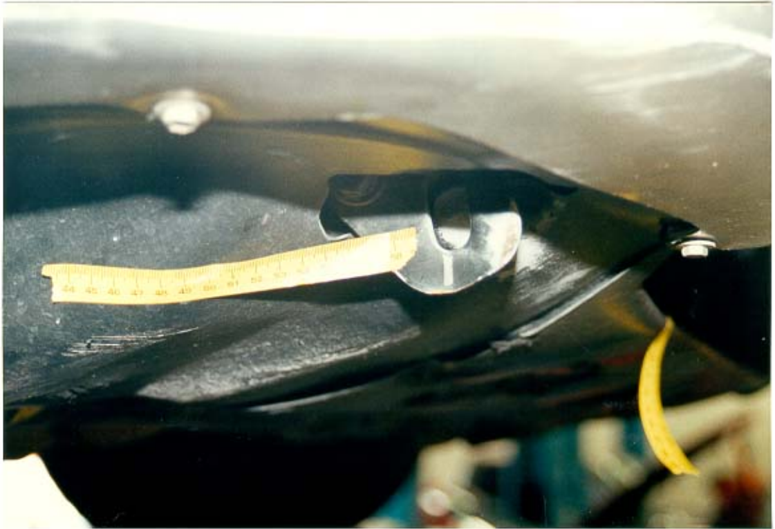
Closeup of damage to underbody
