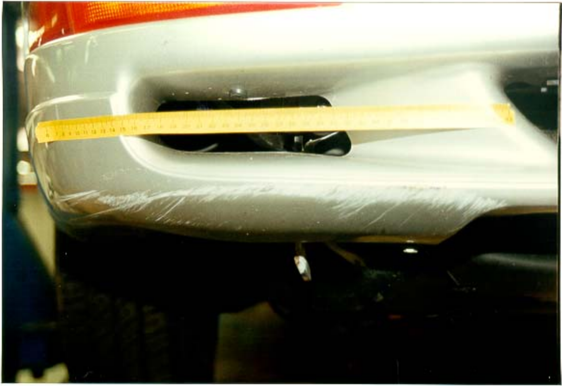
Closeup of damage to fascia
