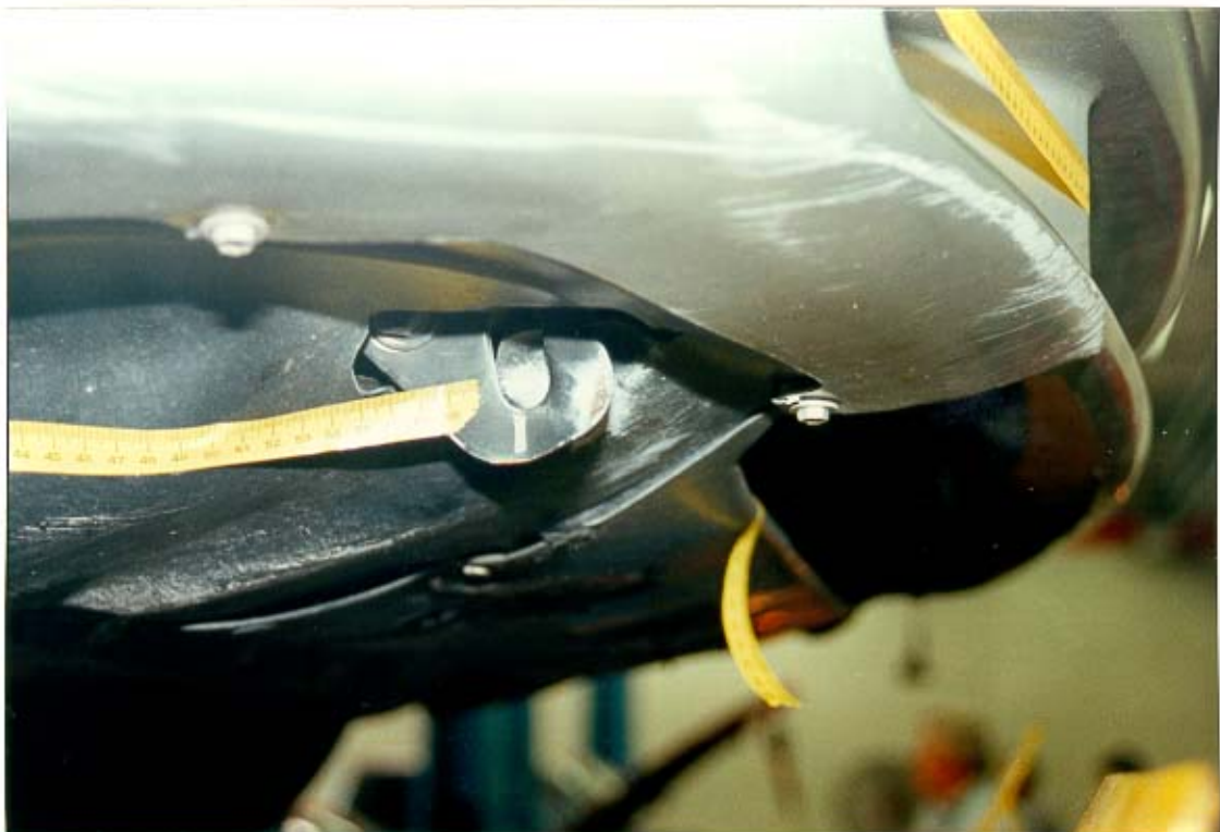
Damage to fascia and tie-down hook
