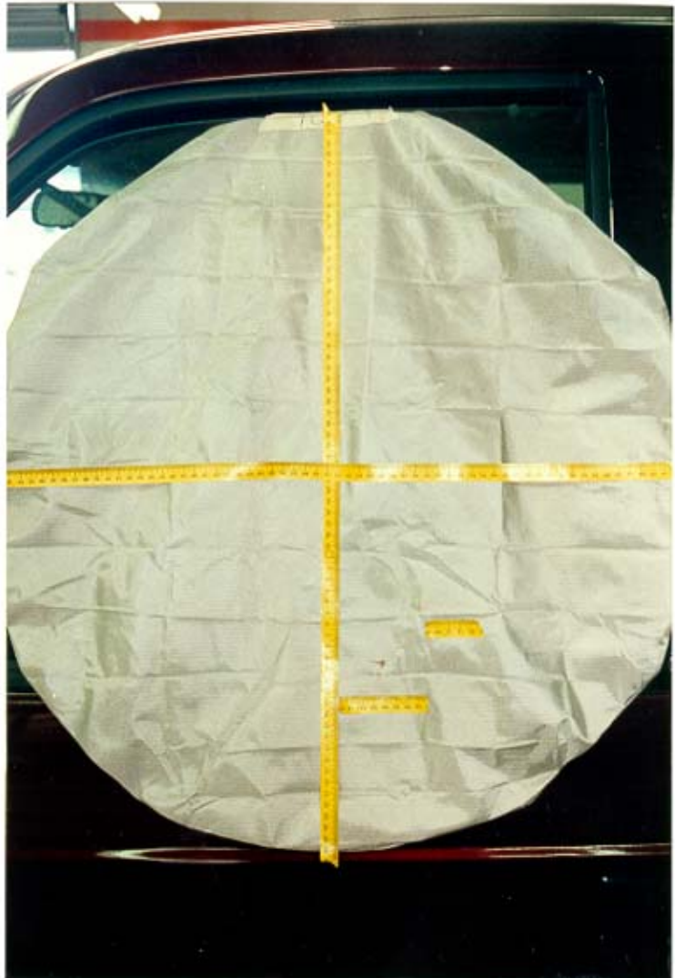
Airbag with blood and scuff highlighted (top of airbag at the top of picture)
