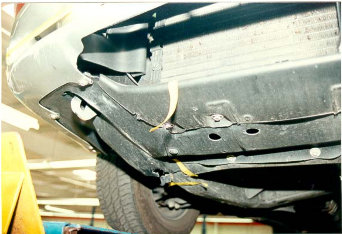
Area of damage to underbody
