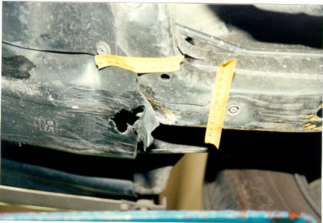
Closeup of damage to right front frame and splash panel
