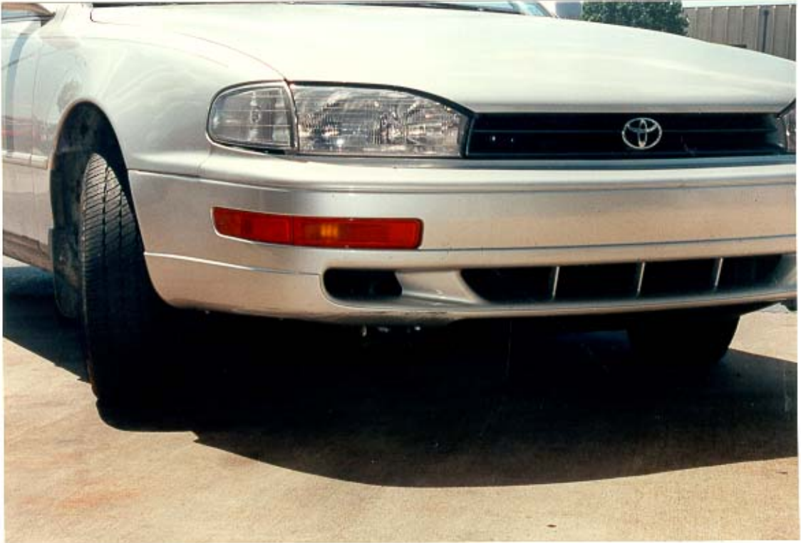
Case vehicle (note scraping on lower right corner of fascia)
