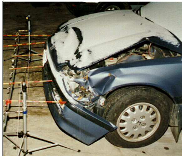
Figure 13: Honda's frontal damage viewed from left along front reference line, with contour gauge present showing deformation (case photo #42)
