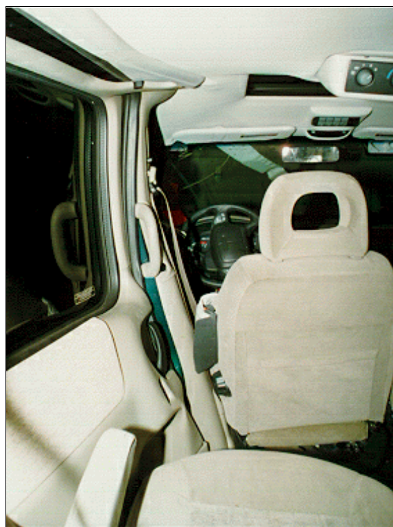
Figure 11: Vertical view from back left seat showing displacement of driver's seat inward and intrusion into left second seating area from left door panel and left "B"-pillar (case photo #32)
