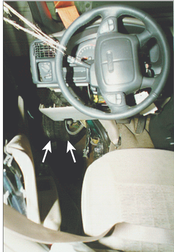
Figure 7: Vertical overhead view of case vehicle's driver seating area from in front of second seat left showing sill intrusion into driver's seating area and displacement of driver's seat toward vehicle's center; Note: arrows mark outline of left front tire (case photo #23)
