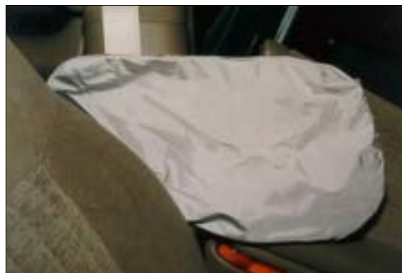
Figure 10: Interior side of case vehicle's deployed, driver, seat back-mounted, side impact air bag showing no apparent evidence of contact (case photo #36)
