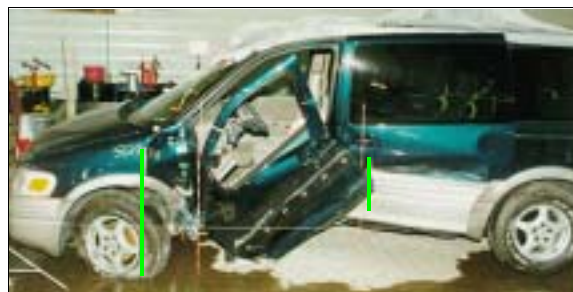
Figure 2: Case vehicle's left side deformation; Note: green lines indicates width of direct damage (case photo #02)
