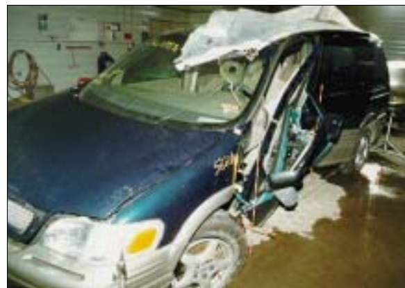
Figure 5: Deformation to case vehicle's left side, viewed from left of front, as a result of impact by front of Honda (case photo #01)
