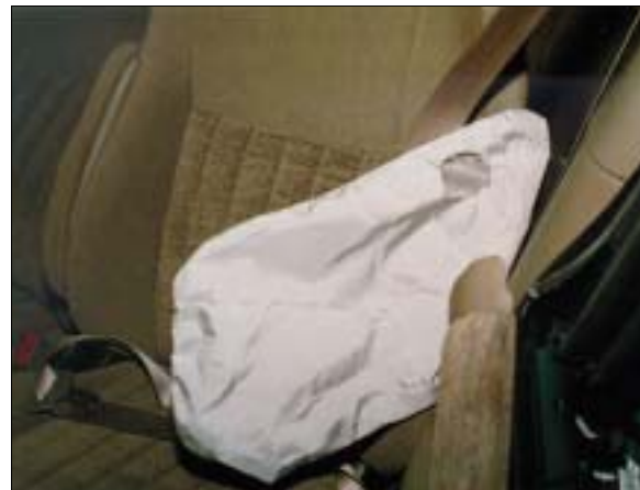
Figure 9: Exterior surface of case vehicle's deployed, driver, seat back-mounted, side impact air bag; Note: vent port was located near top back of air bag's fabric (case photo #37)
