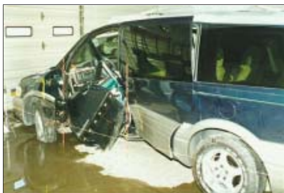
Figure 1: Case vehicle's left side deformation viewed from left of back (case photo #03)
