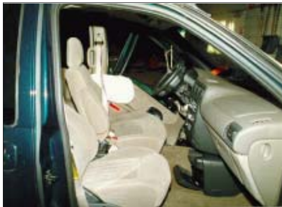
Figure 8: Case vehicle's front seating area showing driver's deployed side impact air bag and non-deployed frontal air bags (case photo #19)
