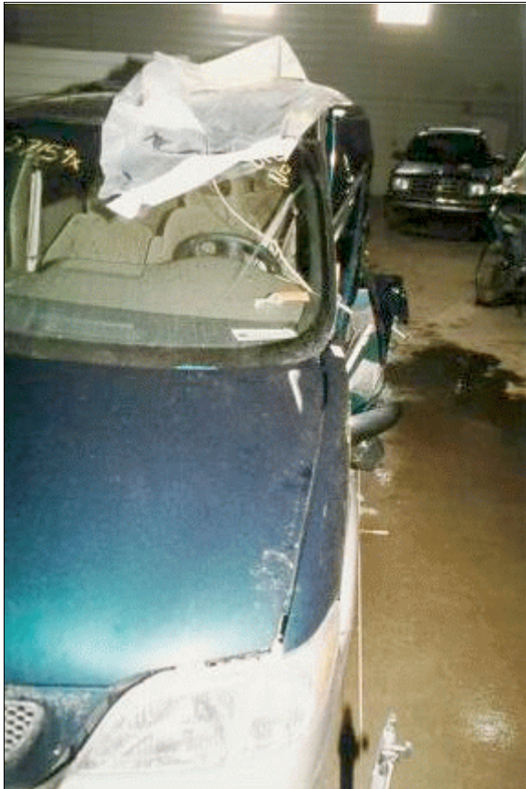
Figure 6: Vertical elevated view along case vehicle's damaged left side showing stringline placement (case photo #12)
