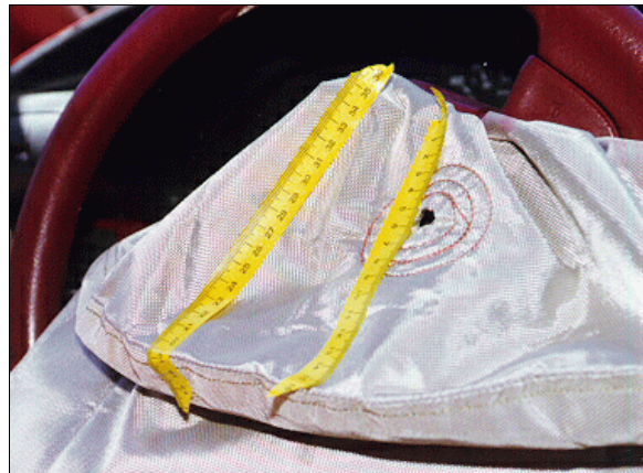
Figure 14: Close-up of skin transfer to backside of case vehicle's driver air bag (case photo #27)
