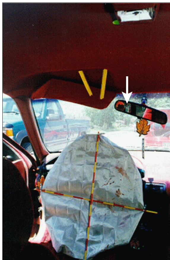
Figure 10: Vertical view of case vehicle's driver seating area showing cracked (arrow) rearview mirror, probable occupant contact to sun visor, and blood evidence on driver air bag (case photo #28)
