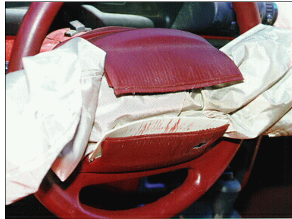
Figure 12: Close-up of cloth transfers deposited on case vehicle driver air bag module's cover flaps; Note: edge of top cover flap struck driver in upper right anterior neck (case photo #22)
