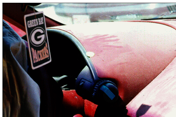
Figure 11: Right hand print deposited on dash by case vehicle's driver when she loaded the steering column during the crash sequence (case photo #31)
