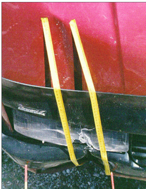
Figure 9: Overhead close-up of deformation to case vehicle's front right bumper, bug deflector, and hood from impact with guy wire (case photo #16)
