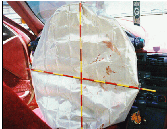
Figure 13: Case vehicle's driver air bag with blood evidence to bottom half; Note: steering wheel turned 90 degrees counterclockwise (case photo #25)
