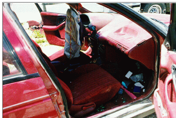
Figure 8: Case vehicle's front seating area, view from right front door, showing deployed driver (only) air bag (case photo #33)
