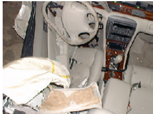
Figure 9 Another overhead view of the left side intrusion looking from the rear of the vehicle forward
