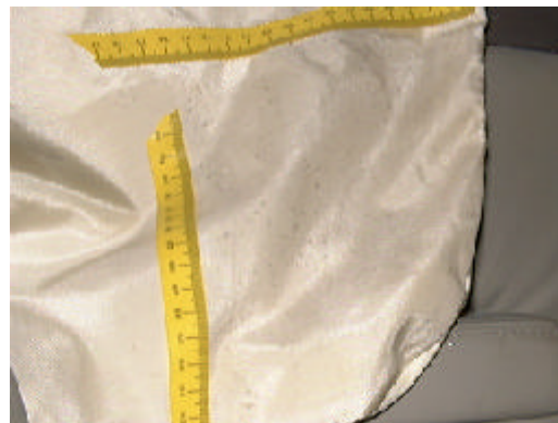
Figure 6 Close-up view of the fabric transfer from contact with the fabric covered lower left B-pillar during the air bag expansion sequence and located along the lower inboard leading area of the side impact air bag surface
