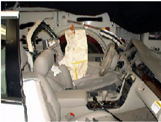
Figure 5 Lateral view of the front seat row of the Cadillac showing the “J” design left front side impact air bag
