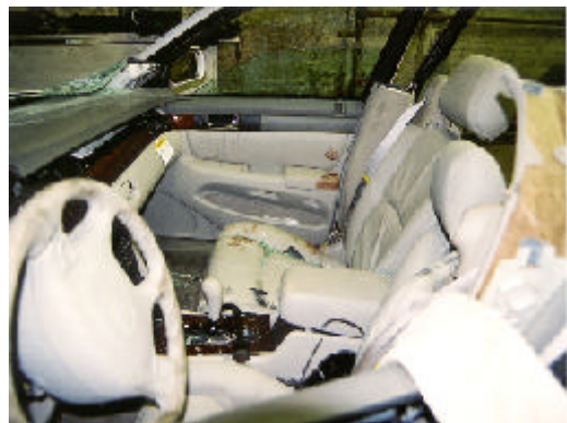
Figure 7 View of the bodily fluid transfer on the front right door armrest and door panel from contact by the driver’s head
