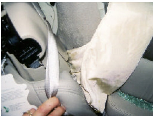
Figure 17 View of the top outboard aspect of the front left seat back support partially showing the air bag deployment area
