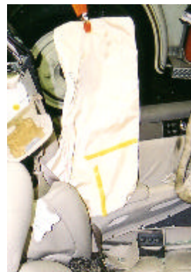
Figure 18 View of the left front side impact air bag
