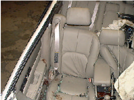
Figure 10 View of the front right seat back support showing the restraint tower incorporating the head restraint, manual belt restraint, and side impact air bag located along the outboard surface of the seat back support
