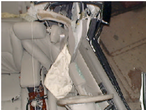
Figure 8 Overhead view of the driver’s seat and the left side intrusion looking rearward from the front of the Cadillac
