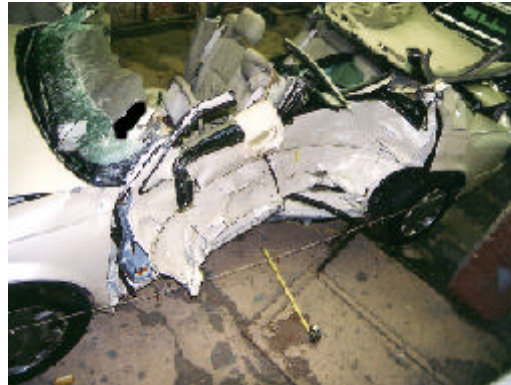
Figure 4 View of the left side impact damage to the Cadillac
