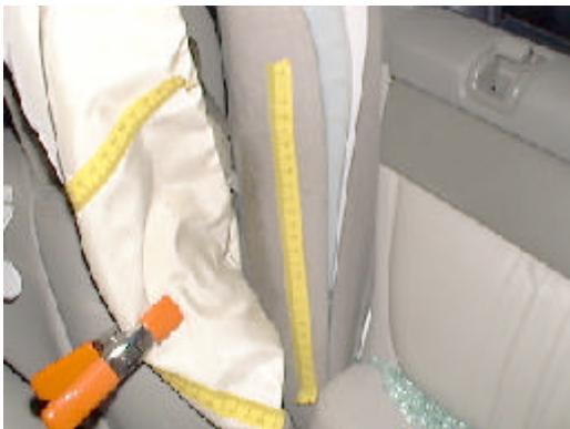
Figure 12 View of the abraded area along the lower left B-pillar from contact by the expanding left front side impact air bag
