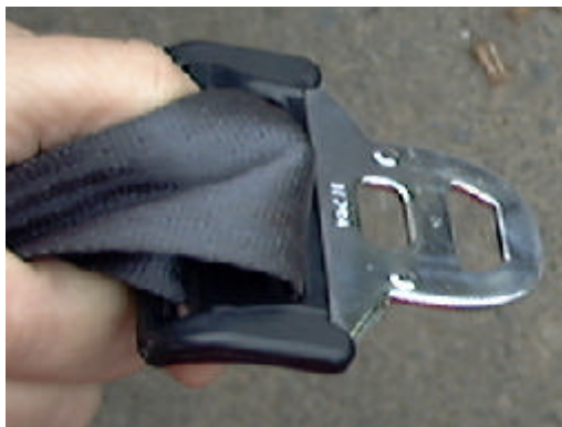
Figure 16 View of the latch plate for the front left 3 point manual lap and torso restraint belt
