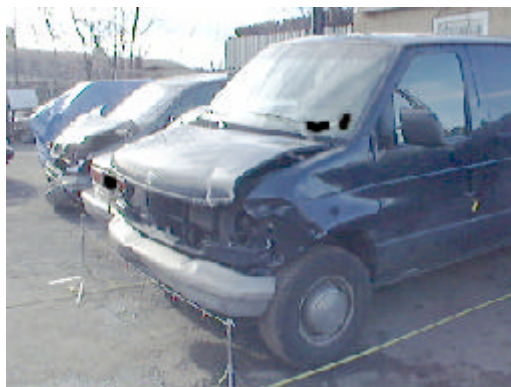
Figure 14 Left corner view of the impact damage to the frontal plane of the 1994 Ford Econoline cargo van
