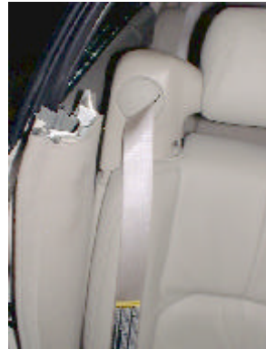
Figure 11 Closer view of the adjustable portion of the restraint tower
