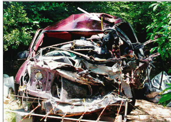
Figure 1: Case vehicle's frontal deformation from impact with Mack truck; Note: direct contact (yellow tape & arrow) to roof near left "A"-pillar (case photo #02)
