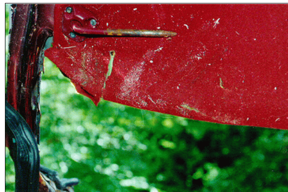
Figure 7: Close-up of skin and hair on case vehicle's roof/front header from contact by driver's head and face; Note: driver's sun visor has been completely torn away from its pivot bar (case photo #22)
