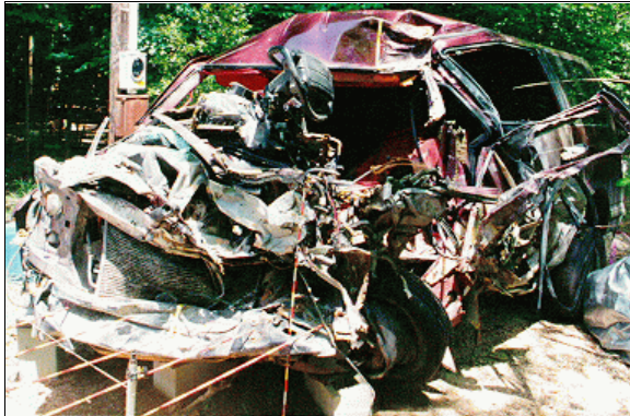
Figure 2: Extensive deformation to case vehicle's front and left side from impact with Mack truck, viewed from left of front (case photo #06)
