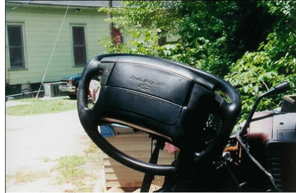
Figure 8: Case vehicle's non-deployed driver air bag (case photo #18)
