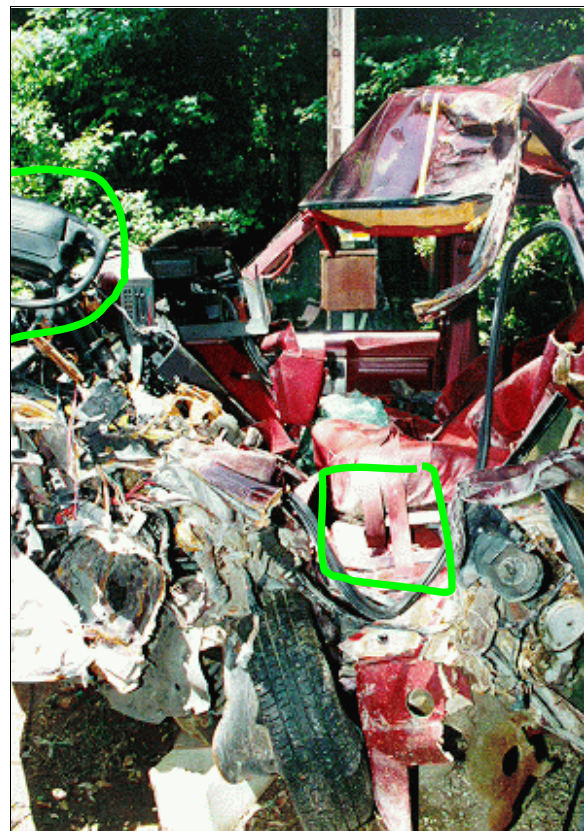
Figure 9: Case vehicle's driver seating area viewed through what once was the driver's door; Note: cut seat belts and twisted steering wheel with non-deployed driver's air bag (case photo #15)
