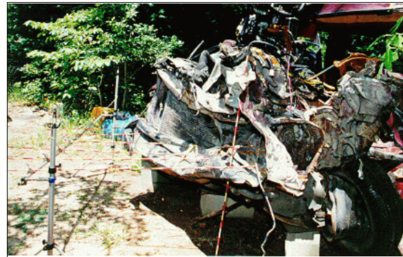
Figure 4: Reference line view from left of deformation to case vehicle's front left (case photo #05)
