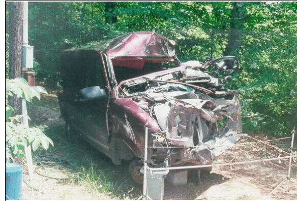
Figure 3: Case vehicle's front left damage viewed from right of front (case photo #13)
