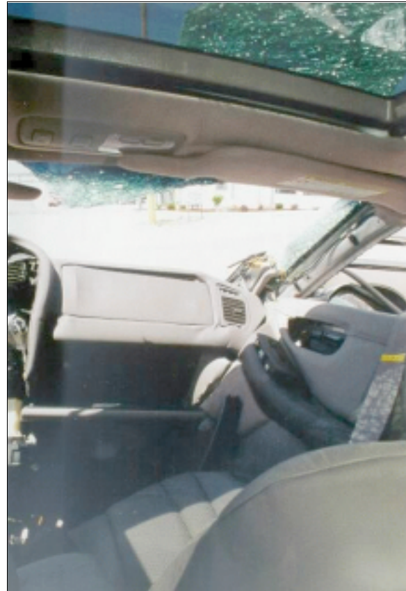
Figure 14: Vertical view of case vehicle's front right seating area showing no obvious contact evidence to right instrument panel or greenhouse area and significant intrusion to seating area from interior surface of right front door (case photo #34)
