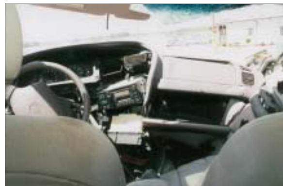
Figure 15: Case vehicle's front seating area showing non-deployed driver and front right passenger air bags and distortion and damage to instrument panel from right side intrusions (case photo #33)
