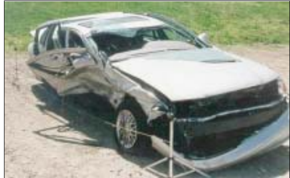
Figure 5: Case vehicle's right side damage from impact with culvert/embankment; Note: stringline adjusted for protruding door (case photo #22)
