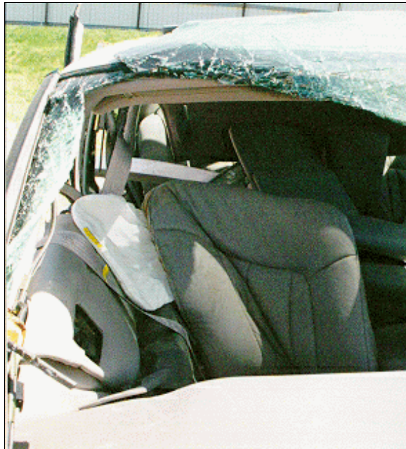
Figure 17: Case vehicle's deployed right front side impact air bag viewed through windshield; Note: intrusion to front right seat and seating area from right front door's interior surface (case photo #35)
