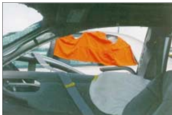
Figure 19: Case vehicle's deployed right front side impact air bag and front right safety belt's webbing showing stretching and blue transfers (case photo #36)
