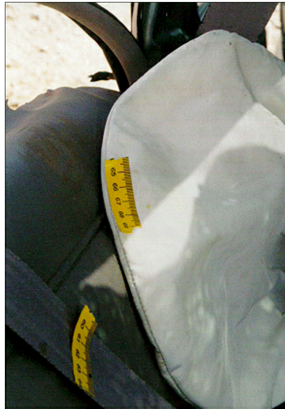
Figure 18: Close-up of interior surface of case vehicle's right front side impact air bag showing unknown fluid dot to right of tape on bag's fabric (case photo #37)
