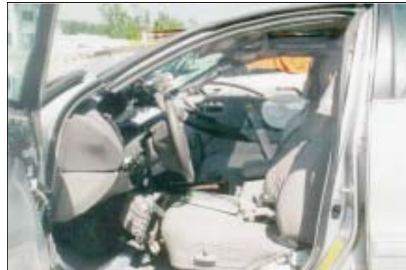
Figure 16: Case vehicle's front seating area showing deployed right front side impact air bag and contact evidence on front right safety belt's webbing (case photo #25)
