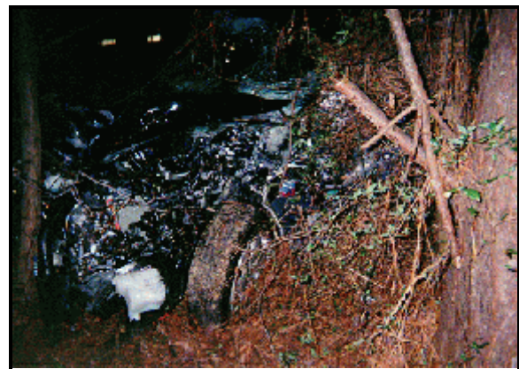
Figure 3: Oblique view of case vehicle's front left damage; Note: exposed left front tire and wheel and position of left front fender (case photo #08)
