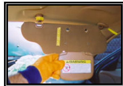
Figure 9. View of damaged front right sun visor
