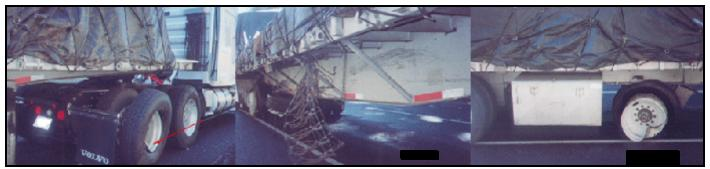
Figure 4. Other vehicle, shows view of damage to rear drive axle, trailer, and front trailer wheel
