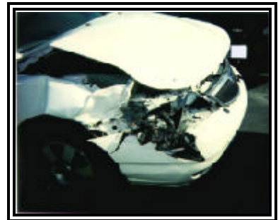
Figure 4. Mercury Mystique right front damage
