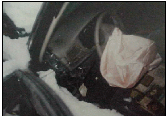
Figure 5: Case vehicle driver's seat area; Note: deployed air bag and damaged steering wheel rim (case photo #13)
