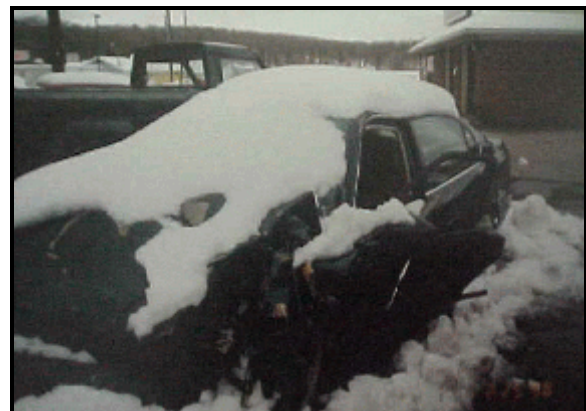
Figure 4: Case vehicle's front left damage from left oblique view; Note: induced damage to left front door (case photo #9)
