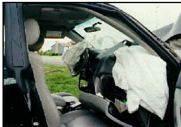
Figure 6: Case vehicle's interior from right front door; Note: steering wheel deformation and deployed air bags (case photo #12)
