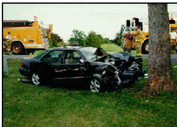
Figure 3: Front right damage to the case vehicle; Note: scrape marks to tree and windshield damage from rear edge of hood (case photo #07)
