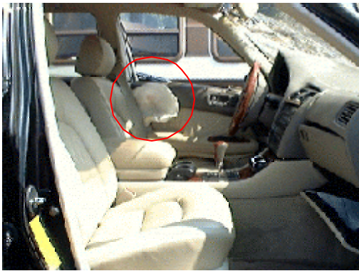
Figure 4 Lateral view of the front seat row of the 1998 Lexus showing the deployed left front side impact air bag
