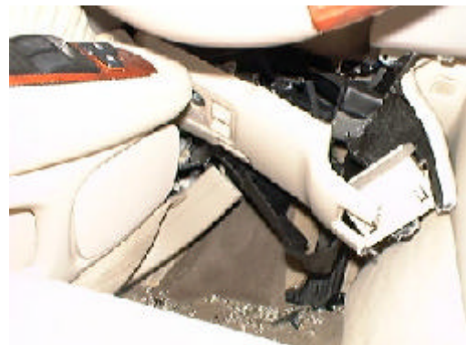
Figure 10 View showing the intrusion of the left side components from the driver's seat looking forward
