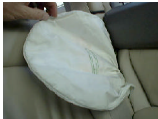
Figure 12 Side surface of the driver’s side air bag facing the left front door panel
