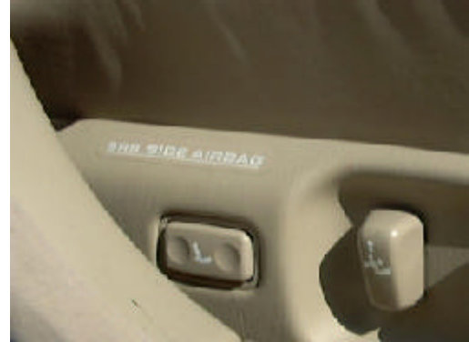
Figure 12 View of the side impact air bag label located above the seat adjustment controls on the outboard surface of the seat
