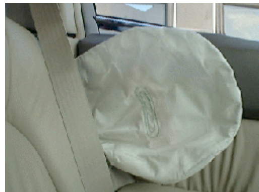
Figure 5 Closer view of the deployed left front side impact air bag
