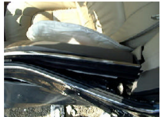
Figure 7 Overhead view of the intrusion in the vicinity of the left front side impact air bag
