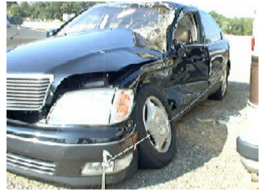
Figure 3 Left front angular corner view of the Lexus illustrating the length of contact and depth of crush
