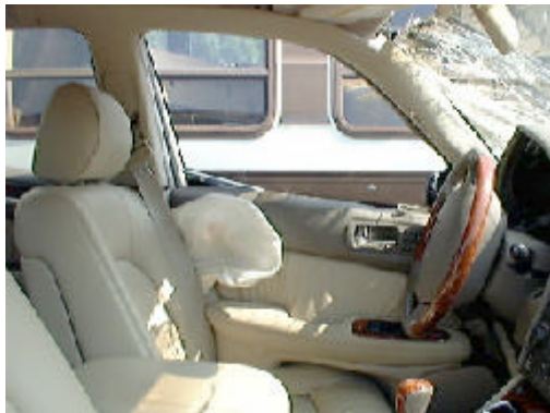
Figure 9 View of the left side of the vehicle illustrating the intruded components
