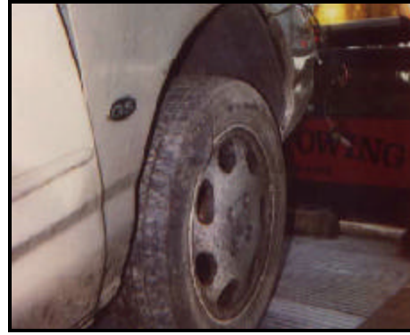
Figure 10. Damaged front, right tire/ tripping force resulting in rollover
