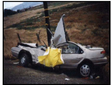
Figure 8. View showing pole impact and Vehicle 1's final rest
