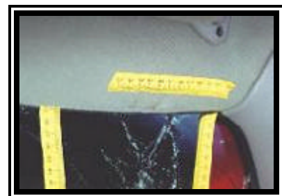
Figure 11. Passenger contact damage to the right windshield header.
