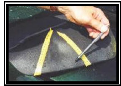
Figure 6. Passenger contact damage to the front right air bag module cover flap.
