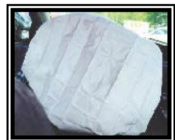
Figure 5. 1998 Pontiac Grand Prix redesigned driver air bag.
