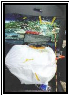
Figure 7. 1998 Pontiac Grand Prix redesigned passenger air bag.
