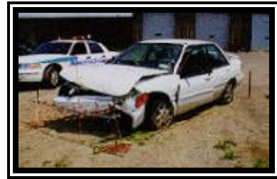
Figure 3. Frontal damage to the 1995 Ford Escort LX.
