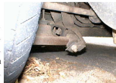
Figure 10. Rotated control arm bushing mount.
