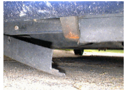
Figure 9. Abraded engine mount and the fractured air deflector.
