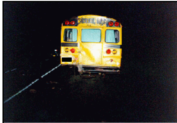
Figure 6: Vehicle #2's rear plane damage; Note: damage limited to left third of rear plane (case photo #10)
