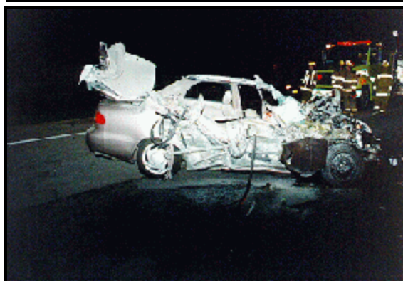
Figure 4: Case vehicle's top and right side damage; Note: damaged hood, windshield, and roof areas (case photo #08)
