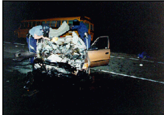
Figure 3: Case vehicle's front damage; Note: roof pushed back over trunk (case photo #04)
