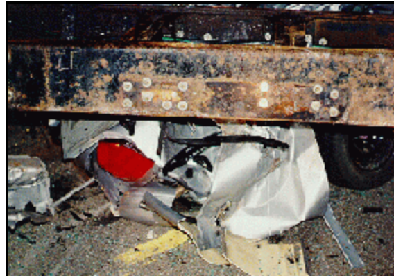
Figure 3: Southeastward view of case vehicle's right rear corner under vehicle #1's right frame rail; Note: left frame rail in foreground (case photo #23)
