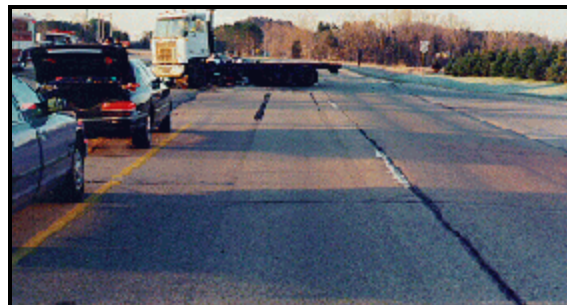
Figure 1: Case vehicle's southbound approach; Note: straight skid marks (case photo #03)
