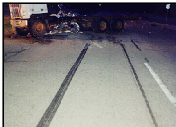
Figure 2: Case vehicle's at-impact deflection marks; Note: case vehicle's at-rest position partially under vehicle #1 (case photo #05)
