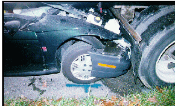
Figure 3: Case vehicle's front right corner contact with vehicle #2's right rear tandem tires (case photo #12)
