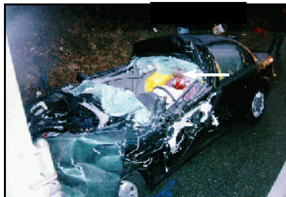
Figure 6: Case vehicle driver’s post-impact position sitting upright but back against his seat back; Note: driver’s face (arrow) is hidden behind the wind-shield which has intruded into front seating area and red spot is blood from the driver’s face which has dripped onto his shirt (case photo #15)
