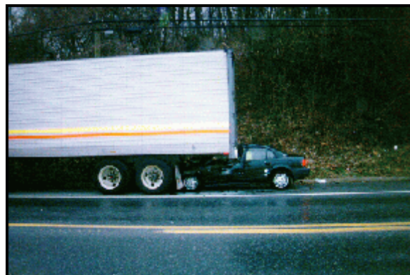
Figure 4: Case vehicle's underride of vehicle #2 showing extent of underride extending almost to "B"-pillars and is offset to back right of semi-trailer (case photo #05)
