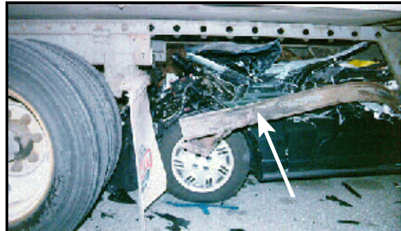
Figure 5: Case vehicle’s contact with vehicle #2’s undercarriage; Note: sheared underride guard channel iron (case photo #06)
