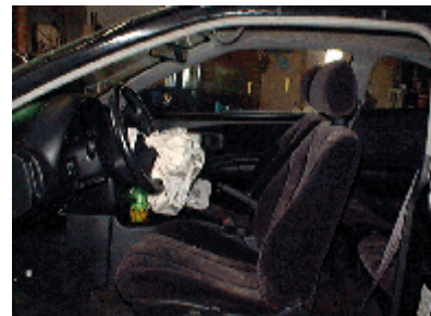
Figure 10. Adjusted seat track position, deployed air bag, and trajectory of the driver.
