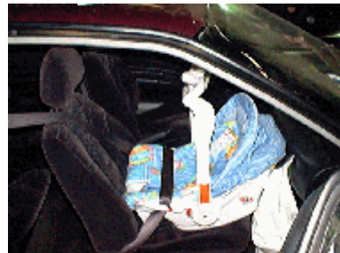
Figure 11. Pre-crash position of the RFCSS.
