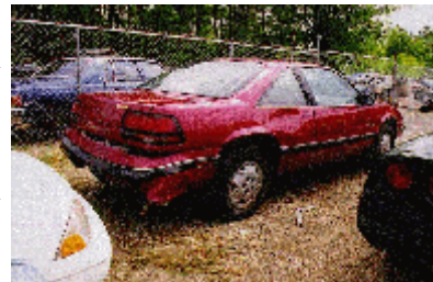
Figure 7. Rear damage to the Pontiac Grand Prix.
