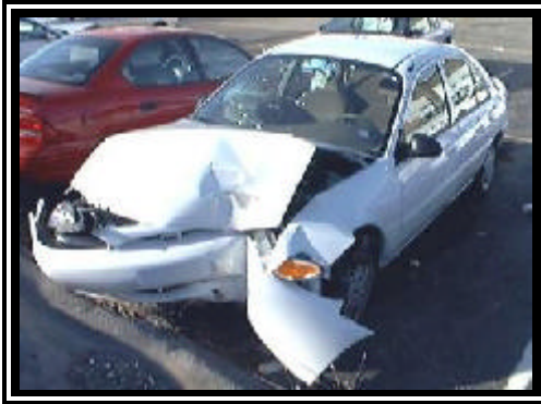
Figure 3. Front left damage to the 1999 Ford Escort SE.
