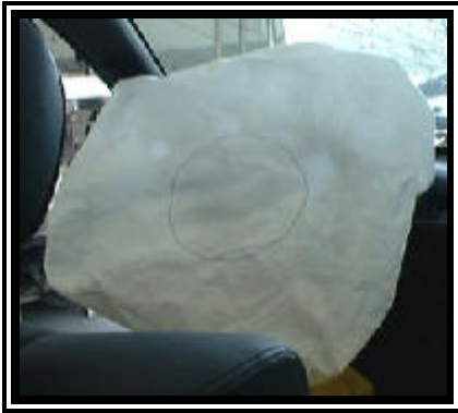
Figure 5. 1998 Toyota Celica GT deployed redesigned driver air bag.
