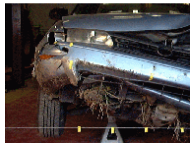
Figure 6. Undercarriage damage to the Corolla.
