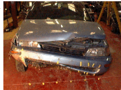
Figure 7. Delineator impact to the bumper fascia.
