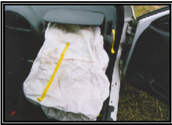
Figure 10: View of the tissue transfers to the top surface of the PAB.
