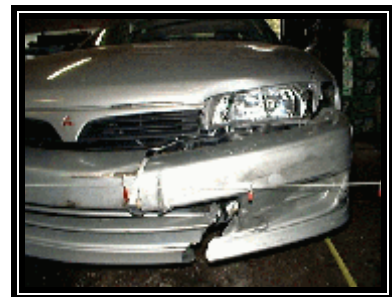
Figure 4 - Close-up view of the direct contact area on the left frontal bumper of Vehicle #1
