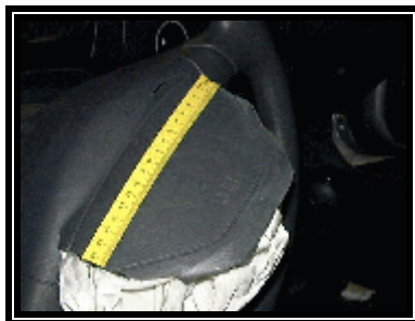
Figure 8 - View of the front left air bag module cover flap showing the fabric transfer along the perimeter of the flap
