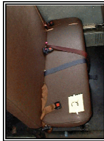
Figure 10 View of row 2 in Vehicle #1 showing the outboard and center lap belts adjusted to the maximum length
