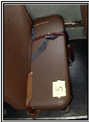
Figure 9 View of row 5 left side in Vehicle #1 showing inboard and outboard lap belt buckles were not visible
