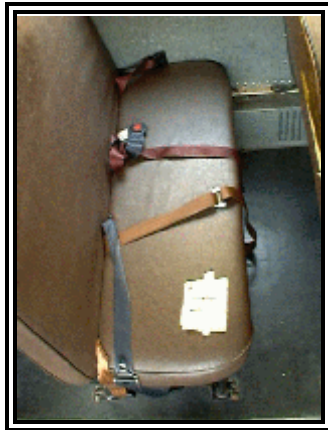
Figure 7 View of lap belts on left side of bus
