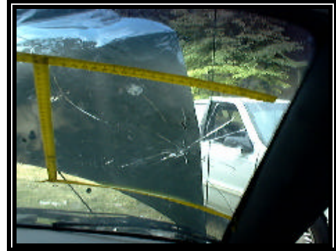
Figure 7: View of the windshield fracture.
