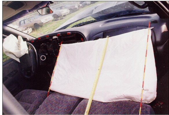
Figure 13: Front surface of case vehicle's deployed front right passenger air bag; Note: a large area of faint skin transfer is present (but not visible) in the upper right portion (case photo #47)
