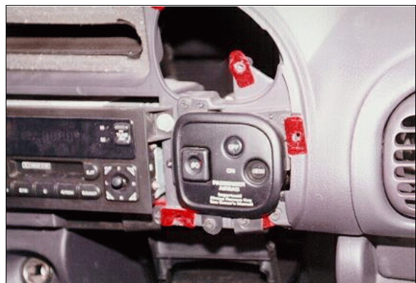
Figure 14: Case vehicle's "On/Off" switch controlling front right passenger's air bag; Note: switch was in ON position (case photo #42)
