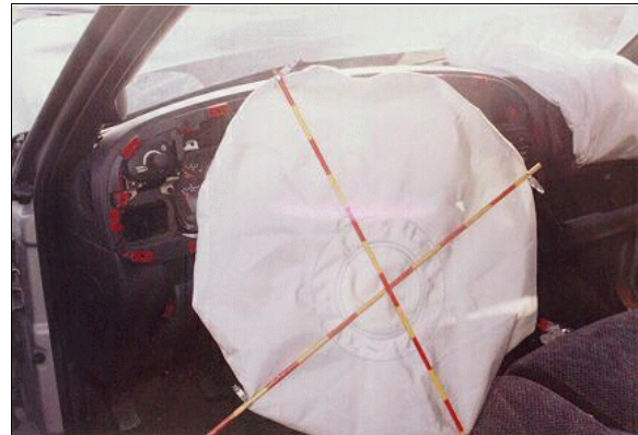
Figure 11: Case vehicle's deployed driver air bag showing no obvious evidence of occupant contact (case photo #37)
