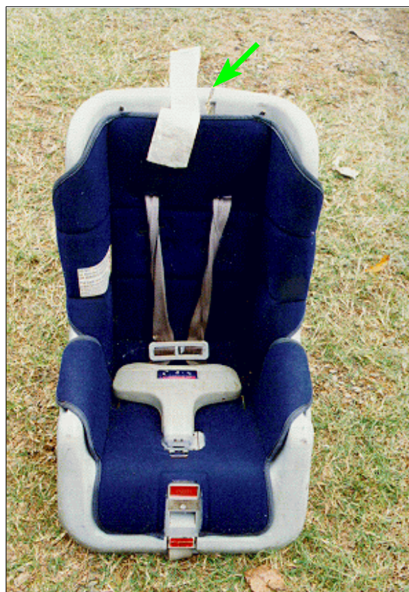
Figure 16: Front of forward facing child safety seat that was secured in case vehicle's front right seating position; Note: crack (arrow) to top of seat (case photo #32)
