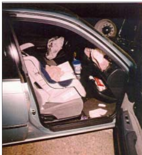
Figure 19: On-scene photo of case vehicle's interior from outside front right door; Note: child safety seat not secured by belt system (case photo #48)
