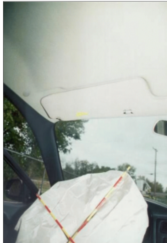
Figure 10: Case vehicle's deployed driver air bag and greenhouse area showing indentation and skin evidence on driver's sun visor (case photo #19)
