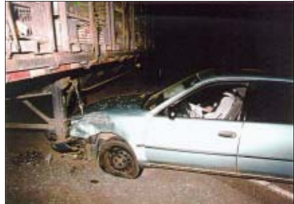
Figure 4: On-scene view of case vehicle at final rest against trailer’s dolly wheels; Note: case vehicle rotated approximately 45 degrees counterclockwise after impact (case photo #45)
