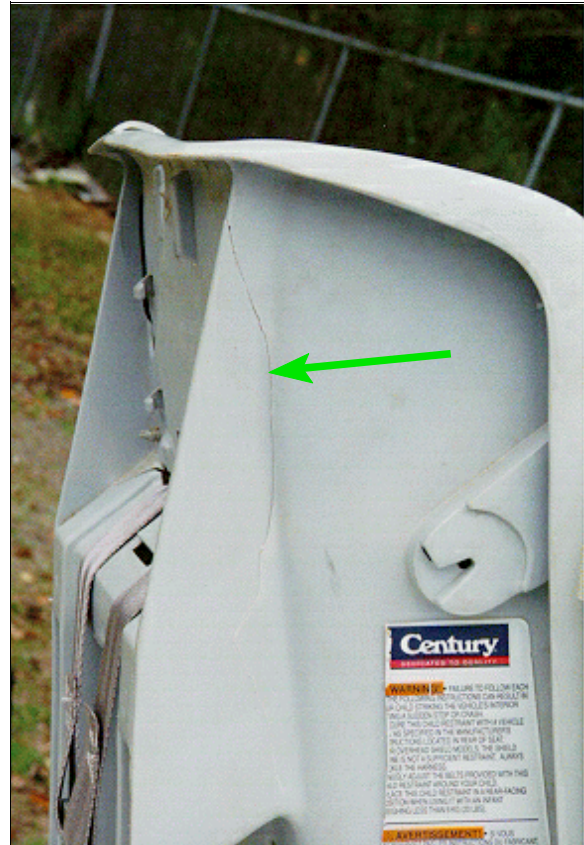
Figure 18: Close-up of right side of forward facing child safety seat secured in case vehicle's front right seating position; Note: crack radiating down side of rear back support bar (case photo #35)
