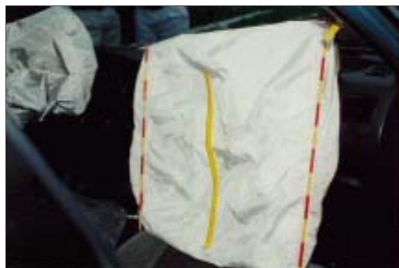
Figure 15: Case vehicle's deployed front right passenger air bag showing skin and grease smears down left side of front portion (case photo #27)
