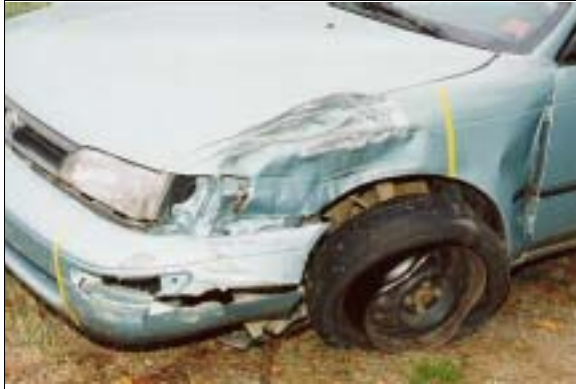
Figure 7: Case vehicle's front left damage viewed from left of front; Note: left front wheel rim snagged during narrow corner engagement (case photo #12)
