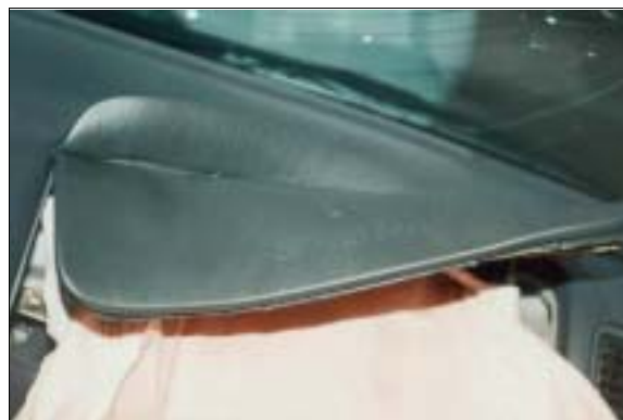
Figure 13: Close-up of evidence on left side of case vehicle's front right passenger air bag module's cover flap from contact with top of forward facing child safety seat (case photo #29)
