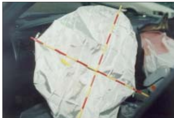
Figure 12: Case vehicle's deployed driver air bag showing contact evidence in right lower quadrant; Note: steering wheel has been rotated clockwise (case photo #25)
