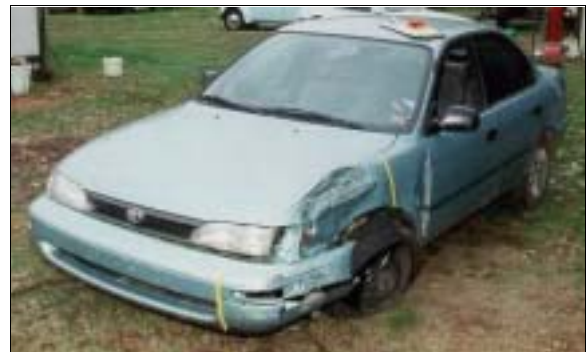
Figure 5: Case vehicle’s very narrow frontal impact with Fruehauf trailer; Note: yellow tape marks beginning (front bumper) and ending (left fender) of direct damage (case photo #08)
