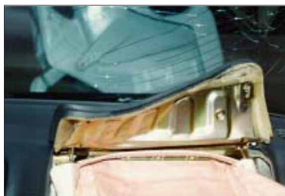
Figure 14: Case vehicle's deformed front right passenger air bag module's cover flap; Note: flap deformed from contact with forward facing child safety seat seen in background (case photo #31)
