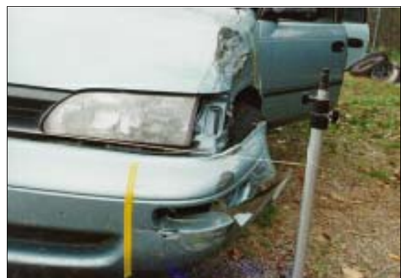
Figure 6: Reference line view down case vehicle’s left side showing narrow direct damage to front left corner (case photo #11)
