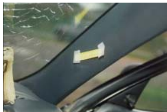
Figure 11: Close-up of scuffing to case vehicle's right "A"-pillar from contact by child safety seat and stress fracture to right side of windshield's glazing (case photo #23)
