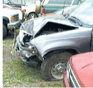
Figure 6. Maximum crush at front left bumper corner.
