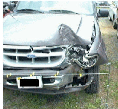
Figure 5. Frontal damage to the Ford Explorer.
