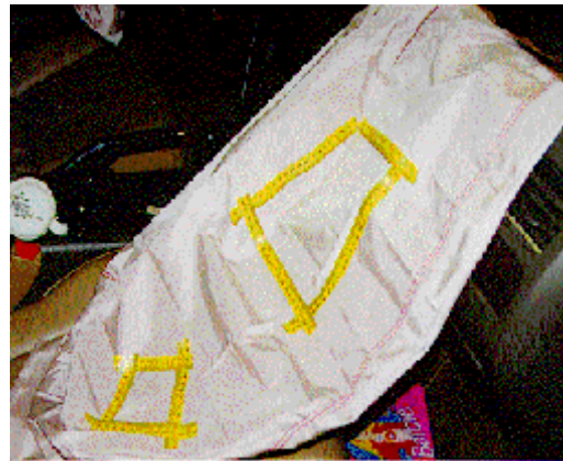
Figure 13- Areas of tissue transfer on the front right air bag of the Acura
