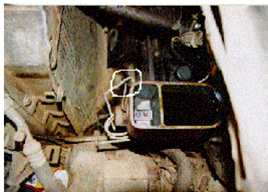
Figure 11- View of the master cylinder from the left side of the vehicle showing the empty forward brake chamber (designated for the rear brakes) and the severed brake line highlighted by the white circle
