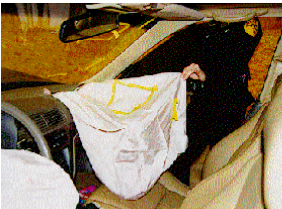
Figure 12- Excursion of the front right air bag in the Acura
