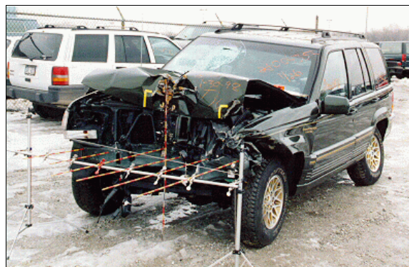
Figure 2: Case vehicle's frontal damage viewed from left of front with contour gauge present; Note: yellow tape on hood near left front wheel indicates direct damage from impact with parked van; yellow tape toward center of hood indicates direct damage from impact with corner of brick building; and angled left rear wheel (case photo #15)
