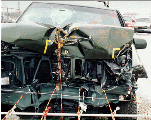
Figure 3: Close-up of case vehicle's front showing deformation from both frontal impacts; Note: yellow tape toward right indicates width of direct damage from impact with parked van, yellow tape near center of vehicle indicates direct damage width from impact with corner of brick building, and slit in windshield near center is from head contact by front right passenger (case photo #12)
