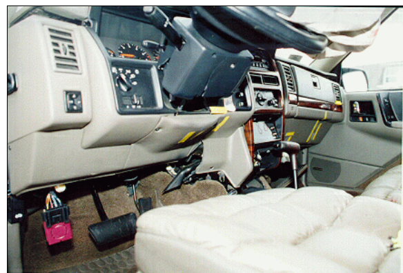
Figure 10: Case vehicle's front seating area showing damage from driver's contact to steering column and knee bolster; Note: damage to front right instrument panel (case photo #29)
