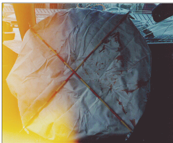
Figure 17: Case vehicle's driver air bag showing blood smears on upper right quadrant; Note: steering wheel rotated clockwise (to right) approximately 45 degrees (case photo #37)
