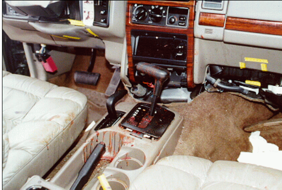
Figure 11: Case vehicle’s center console and floor areas showing blood evidence on console and contacts under right side of steering column and below right instrument panel; Note: distortion to center instrument panel and toe pan intrusions (case photo #38)
