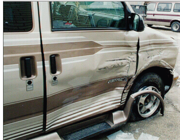
Figure 5: Close-up of damage to Chevrolet's right front door, fender, and wheel from impact by case vehicle's front left (case photo #62)
