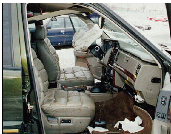
Figure 18: Case vehicle's interior showing deployed driver air bag, close proximity of driver's seat to steering column, and upward movement of steering column (case photo #51)
