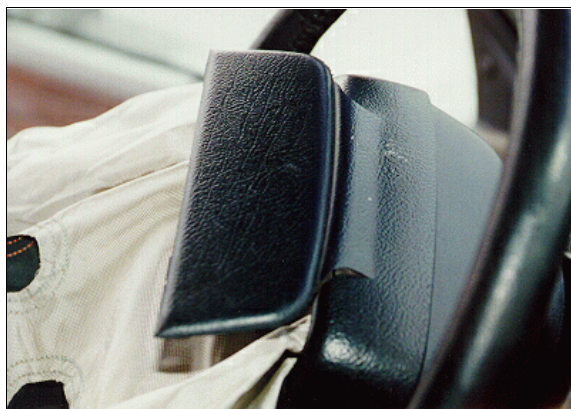
Figure 16: Case vehicle driver air bag module's top cover flap, viewed from front center, showing unknown body fluid splatter on cover flap and air bag's two vent ports (case photo #34)
