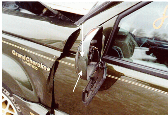
Figure 6: Close-up of case vehicle's damaged left outside rearview mirror from side slap impact with right side of Chevrolet (case photo #19)
