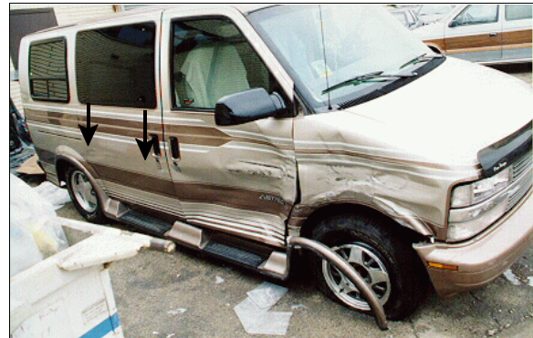
Figure 7: Damage to Chevrolet's right front and narrow area of side slap damage (case photo #63)
