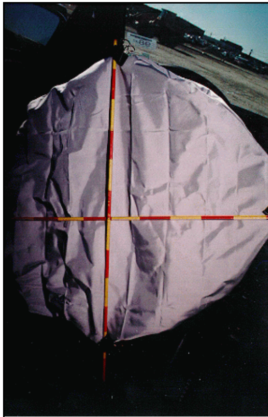
Figure 5: Front surface of driver's air bag (case photo #18)
