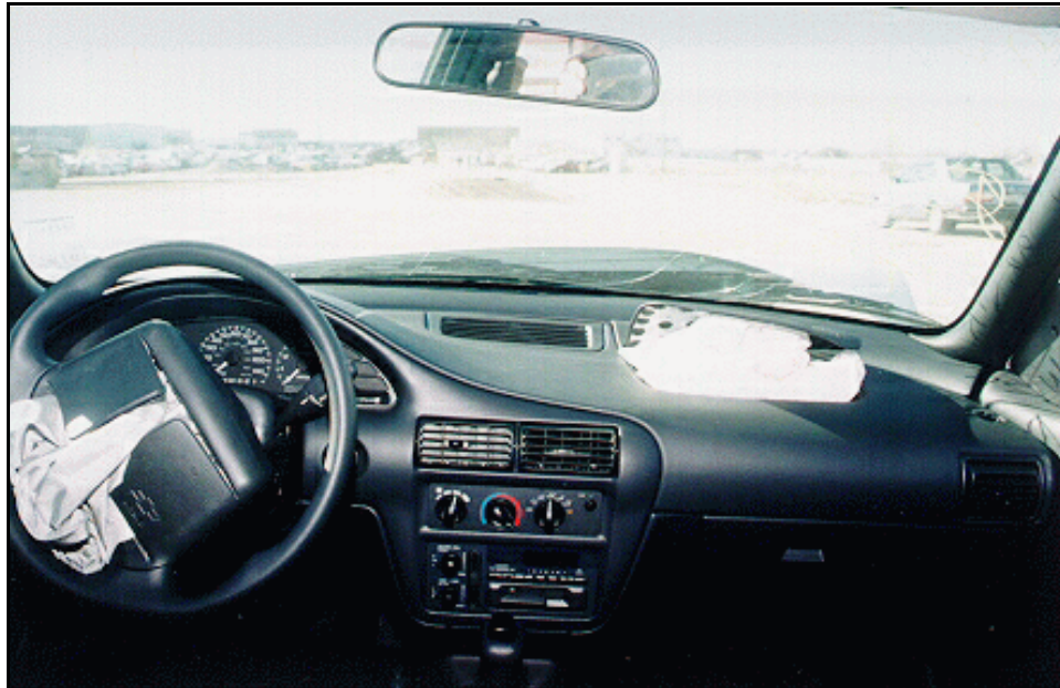
Figure 5: Entire instrument panel; note: front right air bag cover flap (case photo #19)
