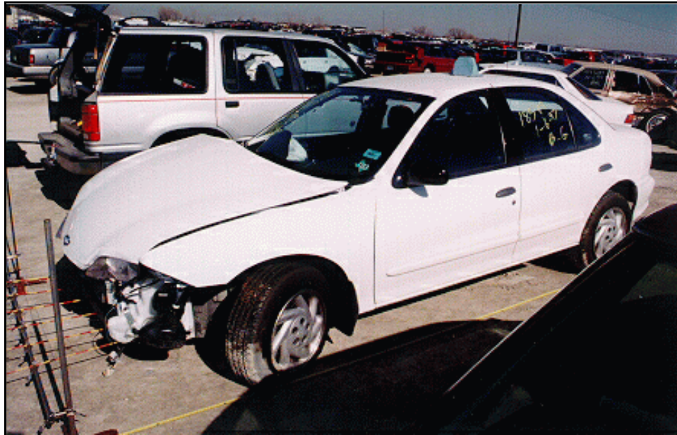
Figure 2: Front and left side of case vehicle; note: bumper and grille assembly torn off by impact (case photo #9)
