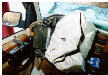
Figure 9. Engagement of the upper module cover flap against the spinner knob.
