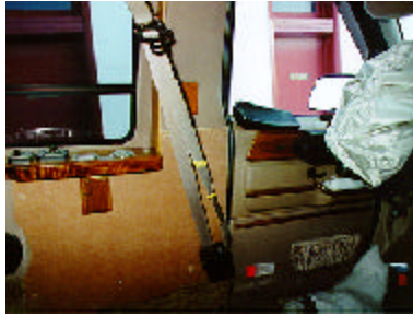
Figure 11. Configuration of the left front manual belt system.
