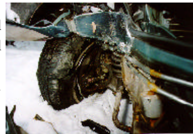
Figure 5. Close-up view of the impact damage to the right front wheel.
