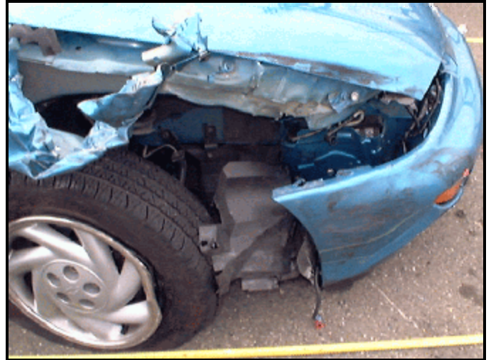
Figure 4. Direct damage, Vehicle 1 (1998 Chevrolet Cavalier)
