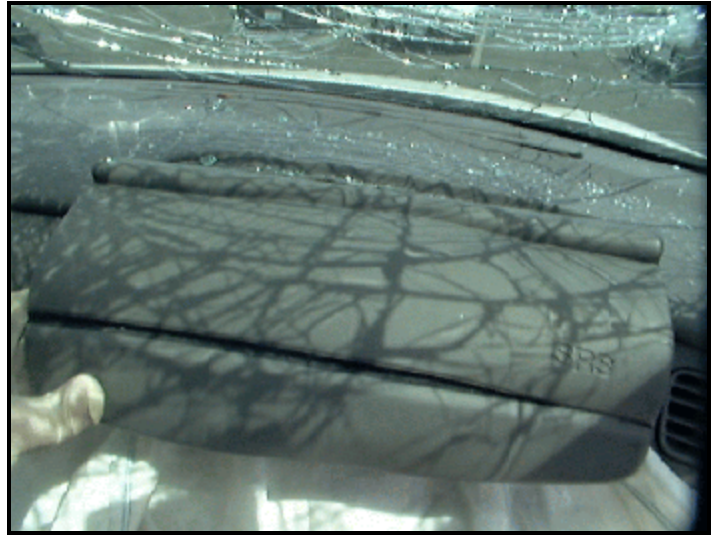
Figure 7. Passenger's air bag cover flap damage
