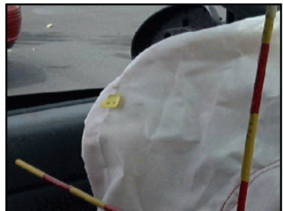
Figure 6. Driver's air bag damage
