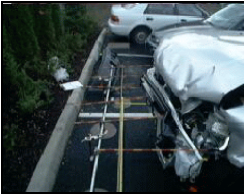
Figure 4. Perpendicular view of Vehicle 1 showing level of crush
