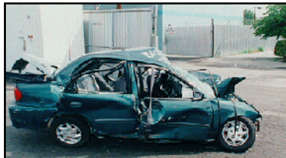
Figure 6: Right side of case vehicle showing curb impact and rollover damage (police photo)
