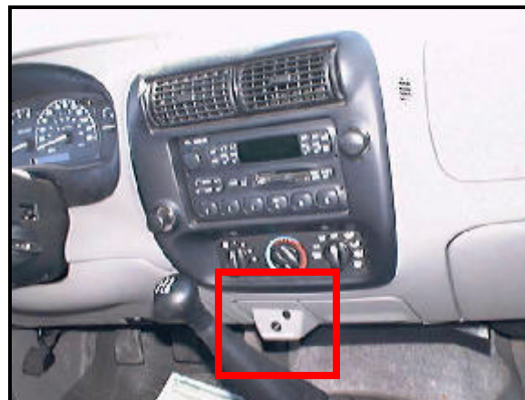
Figure 7. Interior, case vehicle. Box indicates location of passenger's air bag shut off switch.
