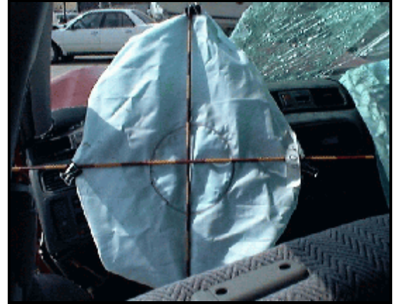
Figure 8. Deployed driver's air bag
