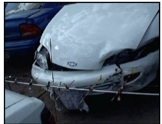
Figure 3. Close-up View of Frontal Damage to Vehicle 1
