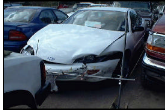
Figure 6. Frontal Primary Impact Vehicle 1 (1998 Chevrolet Cavalier)
