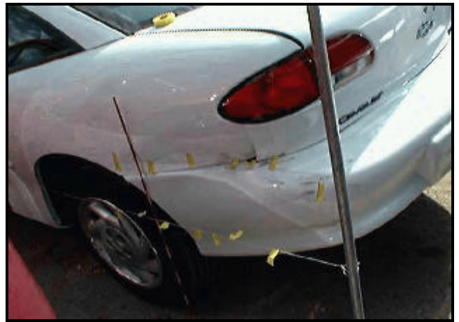
Figure 4. Secondary Impact with Guardrail
