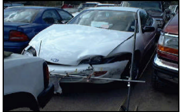
Figure 2. Frontal Deformation to Vehicle 1
