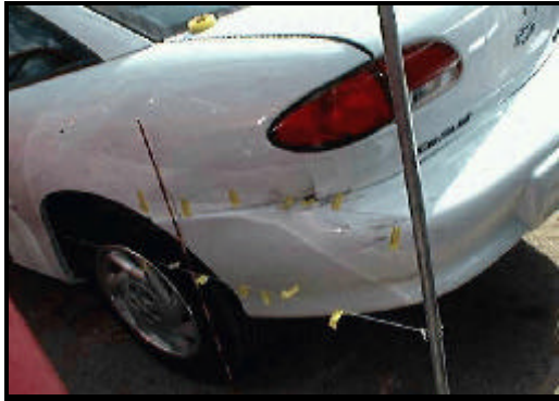
Figure 5. Secondary Impact to Left Quarter-Panel and Bumper
