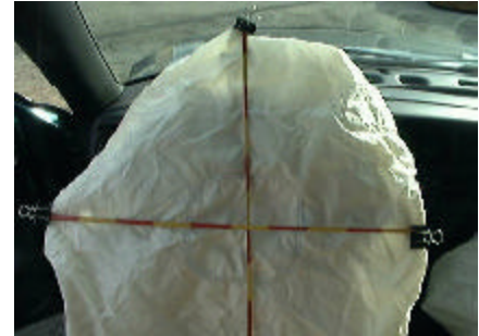
Figure 11. Deployed drivers air bag
