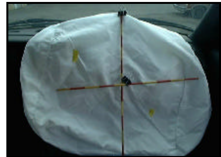
Figure 12. Deployed passenger air bag with occupant contacts highlighted
