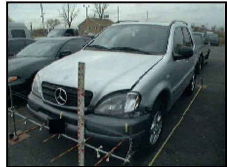
Figure 5. View showing frontal damage to Vehicle 3
