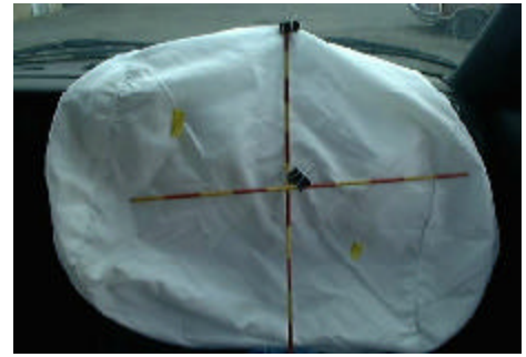
Figure 10. View showing deployed passenger (front, right) air bag
