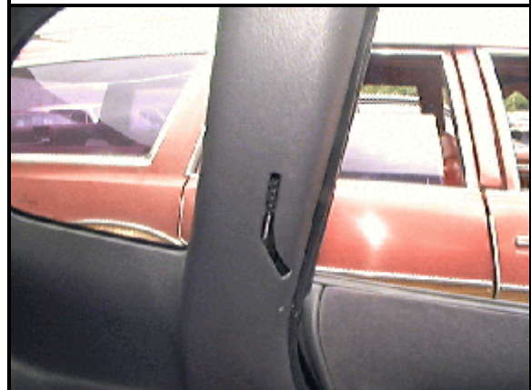
Figure 5: Left B-pillar showing empty slot where cut driver's belt retracted
