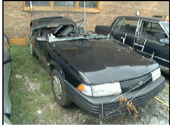
Figure 10: Vehicle #2, front right oblique view; NOTE: pillars cut for extrication of victim
