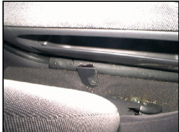
Figure 4: Looking down on driver's door sill, showing cut end of driver's continuous loop belt
