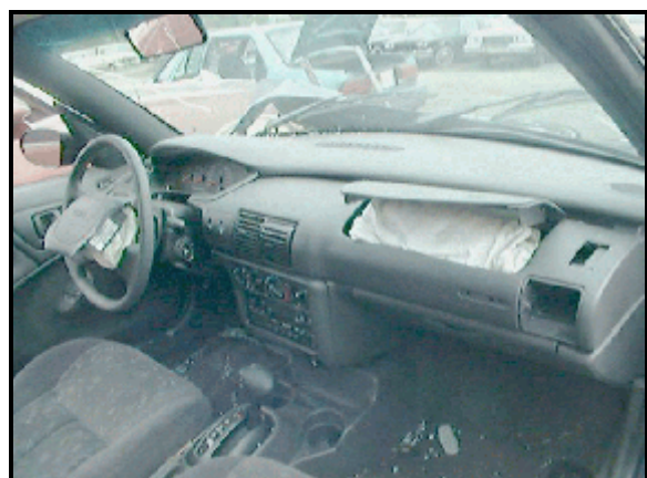
Figure 6: Instrument panel from right, showing driver and passenger air bag cover flaps
